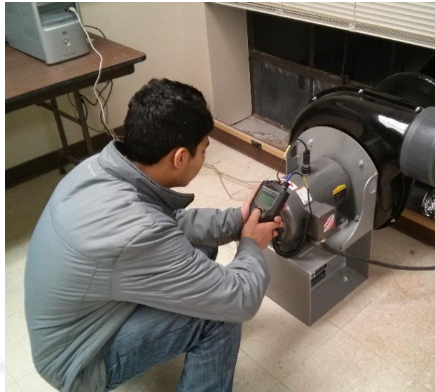
Figure 4.2: Measuring vibration using a vibrometer
