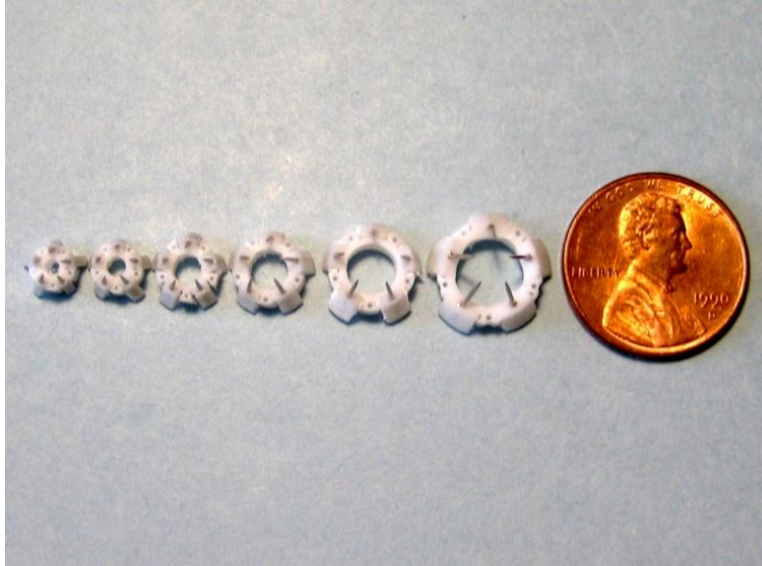
Figure 2.3: Set of five winged couplers for vessels ranging from 1.5-7 mm
