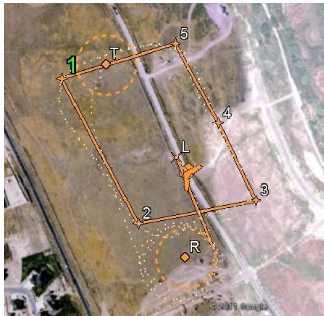
Figure 4.13. Map of the flight path used flight testing as viewed in Virtual Cockpit. Distance between waypoints 1 and 2 is approximately 320 m .
