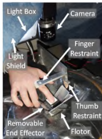
Fig. 4.2. Photo of calibration setup. The camera, mounted on a fixed base, is positioned above the finger, with the light box above and behind the finger. The restraint positions the finger with respect to the flotor, which contacts the fingerpad. To allow the camera to view the scene, the light shield has been partially removed.
