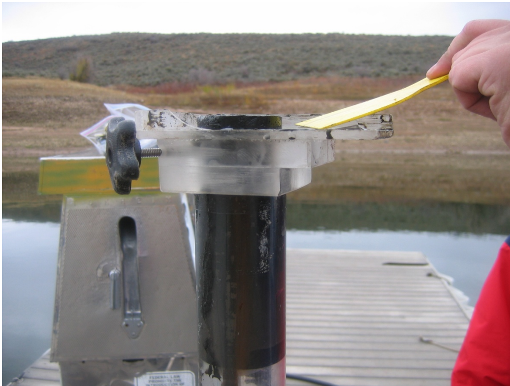
Figure 8: Actual East Canyon Reservoir core and the portable sectioner used to section the cores at 1 cm intervals.
