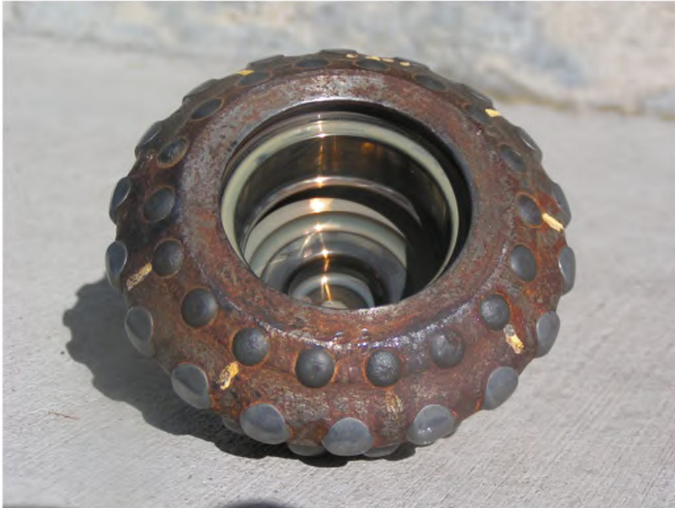
Figure 3.11. A field tested roller cone with GDC inserts in every other position in the heel row (top row in the picture), indicated by the yellow marks.
