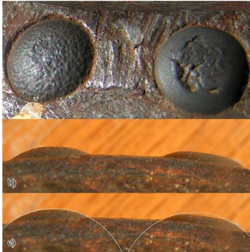
Figure 4.11. Field test results comparing G30 coated drill bit inserts to drill bit inserts coated with an industrial PCD grade. The G30 inserts are on the left. The standard PCD inserts are on the right. a) Comparison of damage to field tested inserts. b and c) Comparison of insert profiles.
