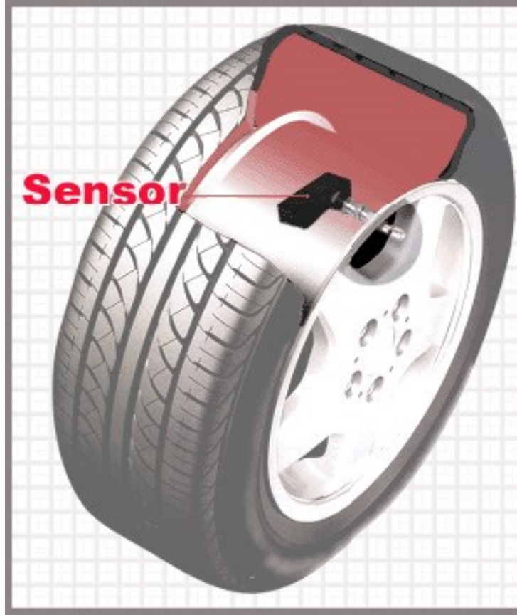
Figure 14. The location of the tire pressure monitor sensor on consumer vehicles. All light vehicles in the United States manufactured after 2007 must be equipped with a TPMS system.
