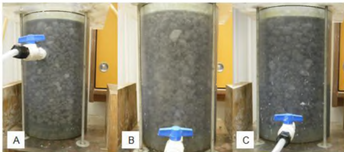
Figure 4.14 Permeability column before testing (A) with C-16 (B) with acid only (C) with C-17.
