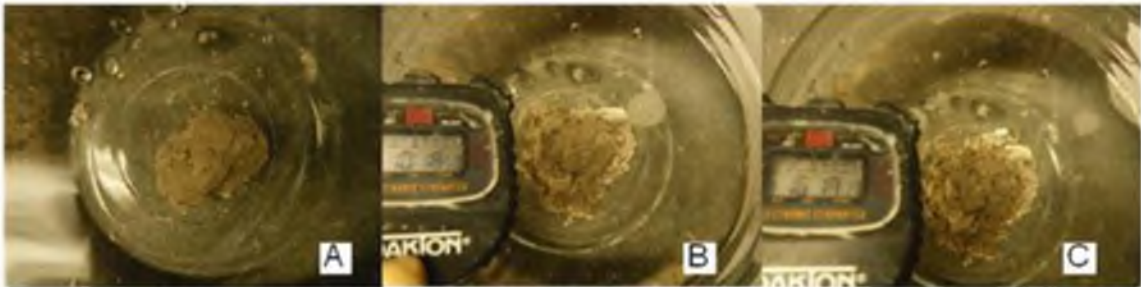
Figure 2.13 TBS test where changes can be seen A) at the beginning B) during the test and C) at the end of the test. The agglomerate can be seen degrading as the test progresses.
