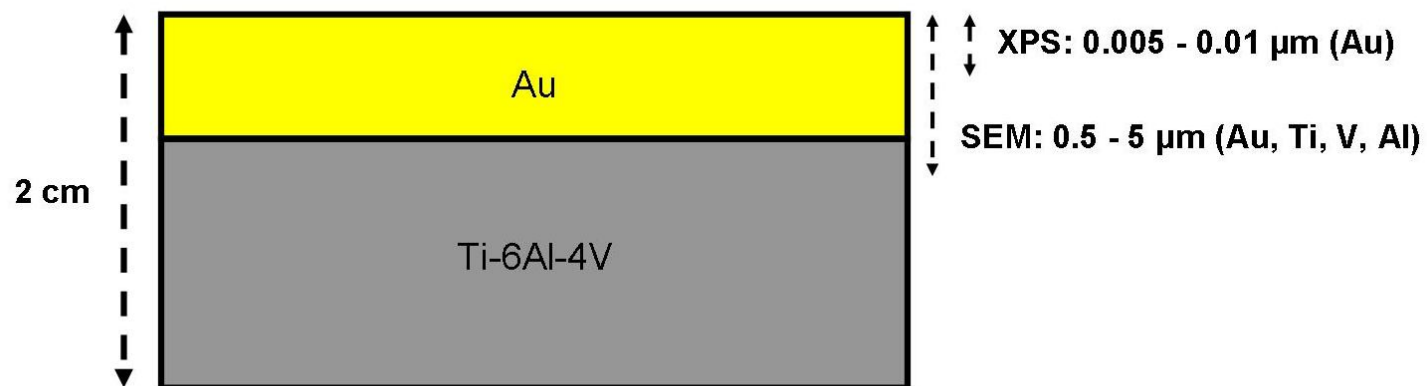
Figure 47: Representative diagram of the anode surface using the XPS and SEM analytical techniques. Note the XPS analytical tool demonstrated only gold on the surface of the electrodes, while the SEM determined the surface to be a combination of gold, titanium, vanadium and aluminum.
