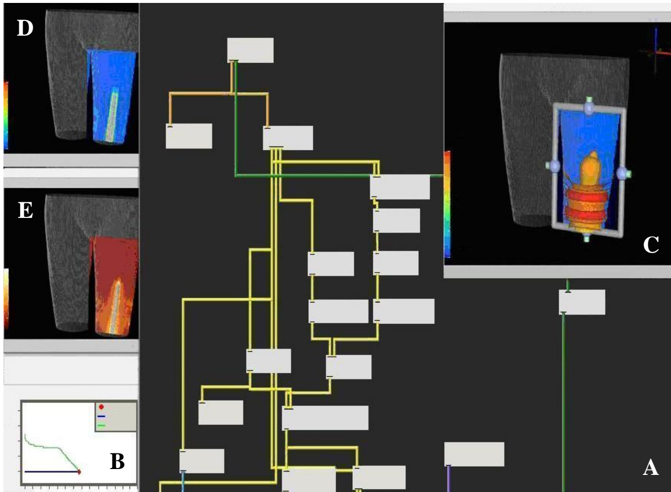
Figure 13: Representative image of a partial network used for inserting model boundary conditions (A), performing iterative solving (B), design electrodes (C) and calculating the electric field (D) and current density (E) at the bone-implant interface.
