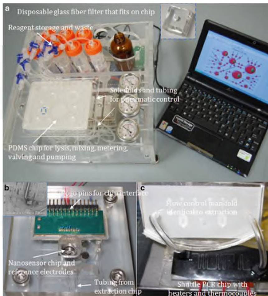
Fig. 2. (a) Prototype of an automated nucleotide extraction platform. The microfluidic system consists of five different components: (i) a disposable microfluidic cartridge containing a glass fiber filter (inset figure); (ii) a PDMS-microfluidic chip for flow control; (iii) microfluidic chambers for mixing, metering, pumping, and reactions; (iv) a pneumatic micropump to deliver the eluted sample to downstream assays; and (v) a vacuum pump to control the on-chip valves. The extraction chip also has provision for thermal lysis and reverse transcription (not shown). (b) Prototype of a test socket for characterization of a carbon nanotube-based electrochemical nanosensor array. The test socket provides both fluidic and electrical interface to the nanosensor chip (inset figure) that detects nucleotide hybridization. (c) Prototype of a shuttle PCR chip with three temperature zones and which is fabricated using polycarbonate lamination. The heaters and thermocouples are shown with a manifold for on-chip fluidic control. The fluidic interface for the extraction system is designed so that it can be readily connected to the downstream assays such as hybridization and PCR.
