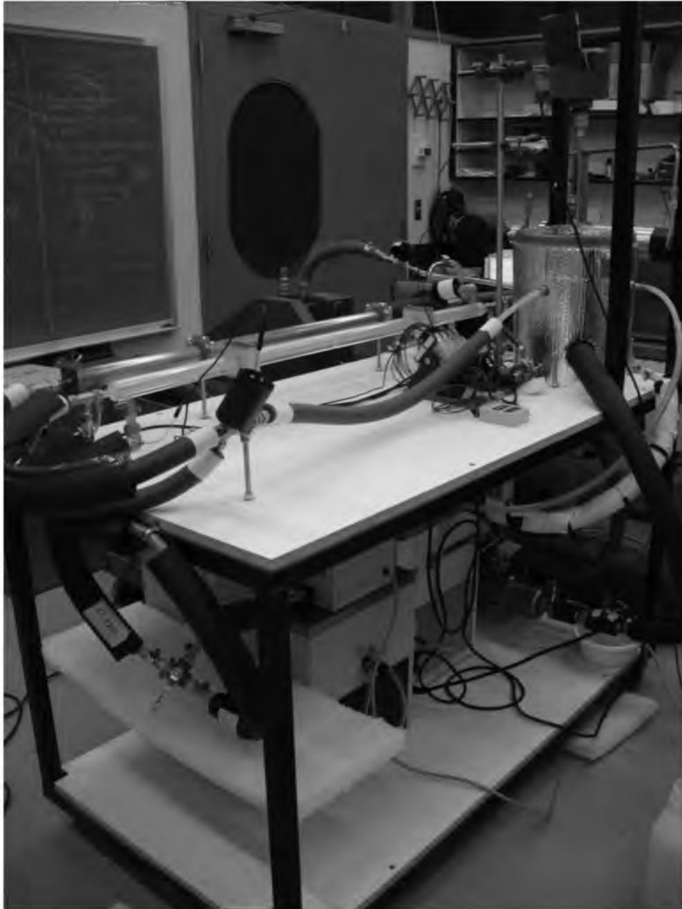
Figure A.7. Rear-view of Flow Loop version 3.0. Coolant valve seen in bottom left; this valve diverts flow between test sections. Progressive cavity Moyno pump seen to the right on the bottom of the cart.
