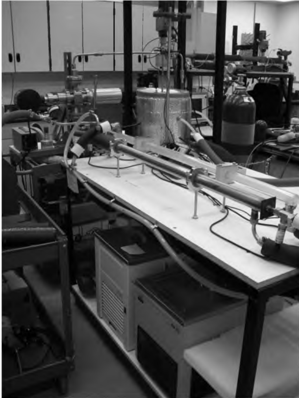
Figure A.6. Flow Loop version 3.0 with both steel and acrylic test sections. A valve at the inlet (further back in the image) diverts flow from one to the other. CantyVision system is seen at the upper left corner, reservoir is just above center, and temperature controllers are on the bottom of the cart.
