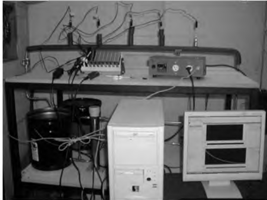
Figure A.1. Flow Loop version 1.0. Two reservoirs for sending and receiving visible to the left. Flow lines proceed from ISCO pump (bottom center-left) up to the left, across through a pipe fitted with transducers, then into the receiving reservoir.
