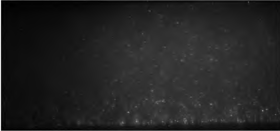
Figure C.135. PIV image of 0.328 psi/s (4.7 Pa/s shear stress) loading case before breakage.
