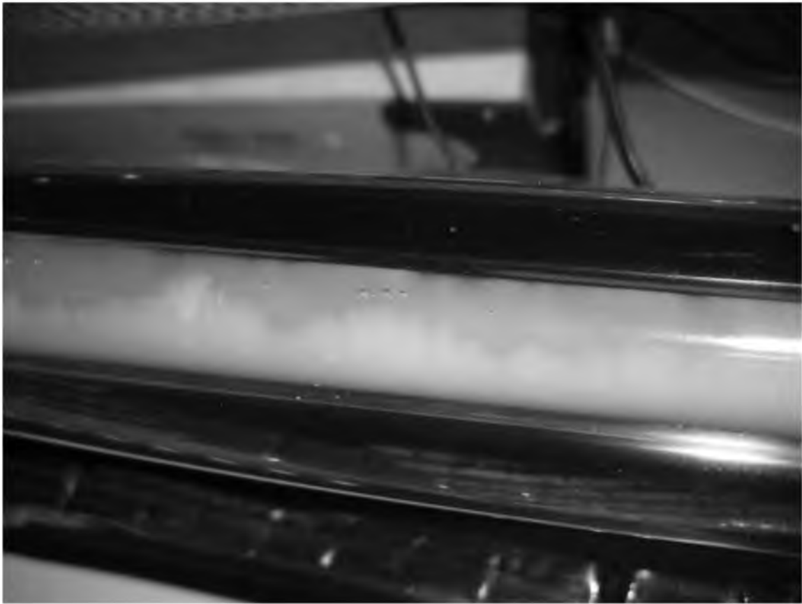
Figure A.4. Visualization of wax deposition forming inside the acrylic test section of FLv2.1.
