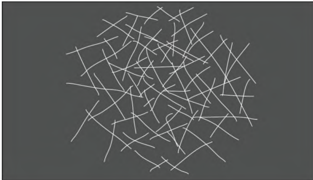
Figure 4.16. Cartoon of natural gel matrix formation with no preexisting crystals. Such a gel matrix features a large number of high quality cross-links between wax crystals.
