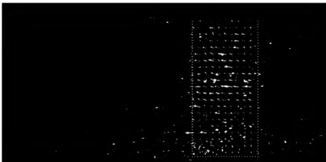
Figure 4.32. Enhanced image of Figure 4.31. Consistent vectors have appeared in the bulk of the gel indicating fracture and flow. No such vectors are seen at the walls (top and bottom of the image) indicating center-core failure.
