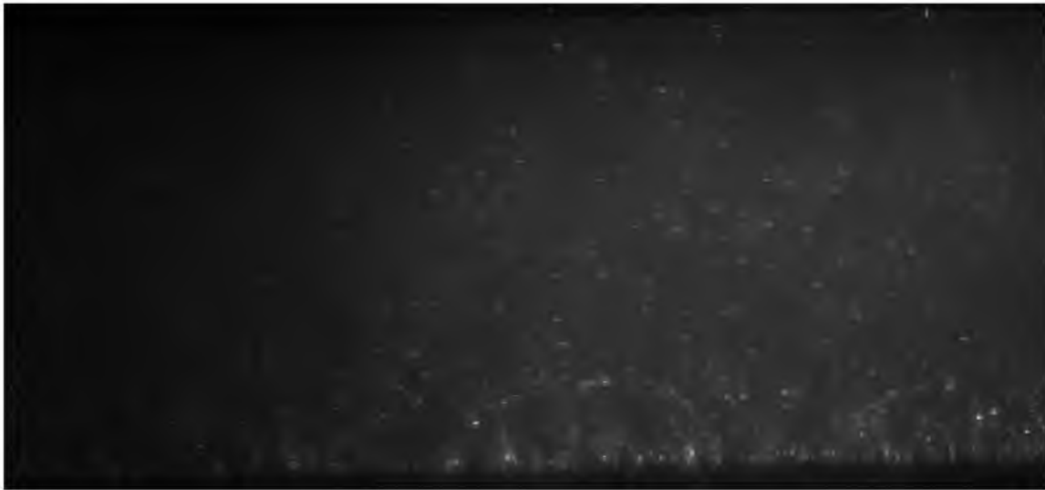
Figure C.136. PIV image of 0.328 psi/s (4.7 Pa/s shear stress) loading case after breakage
