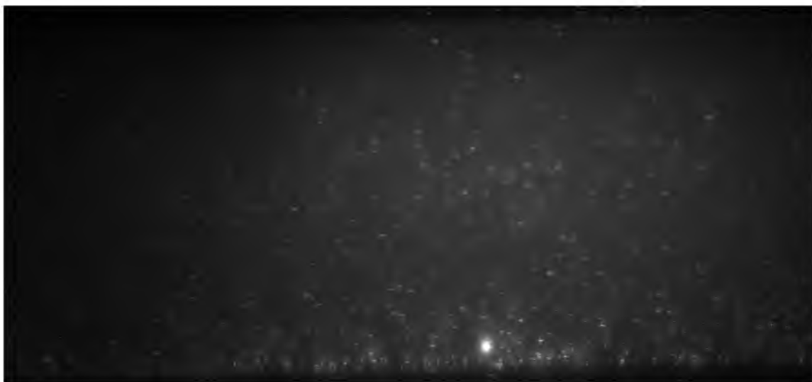
Figure C.126. PIV image of 1.62 psi/s (23.3 Pa/s shear stress) loading case after breakage.
