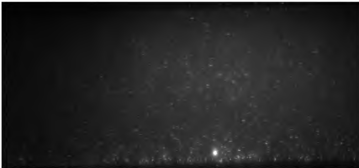
Figure C.125. PIV image of 1.62 psi/s (23.3 Pa/s shear stress) loading case before breakage.
