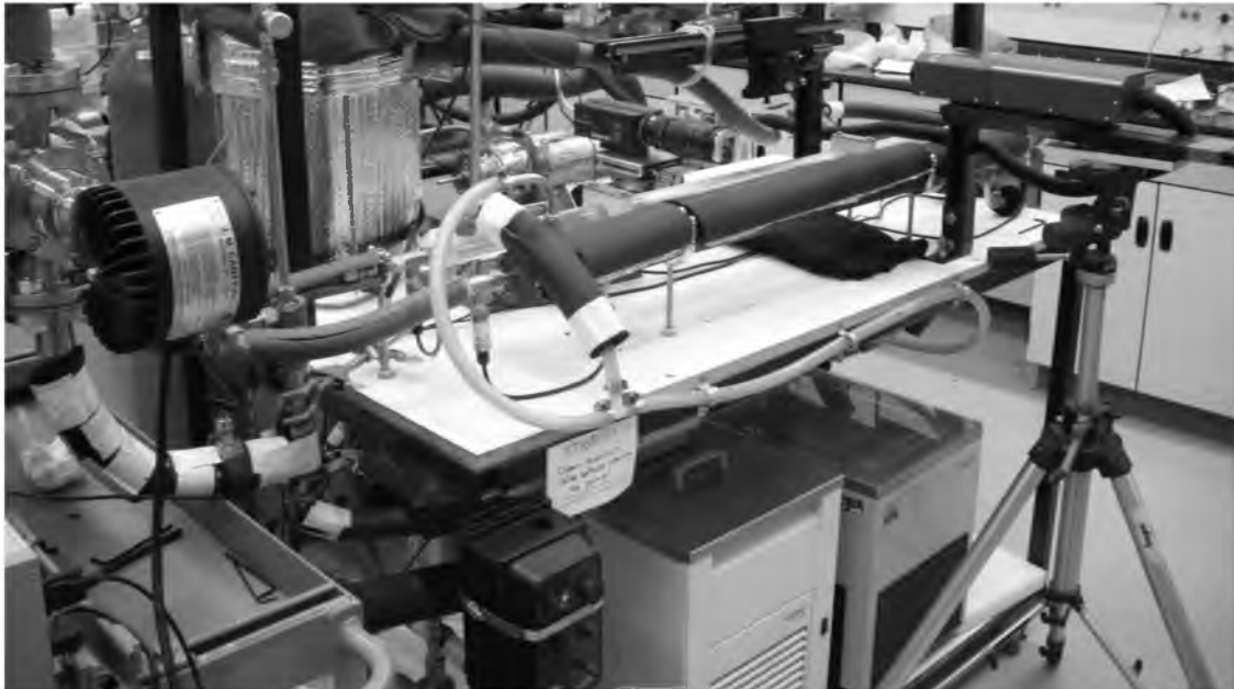
Figure 2.16. Photograph of FLv3.2 showing most of the experimental flow lines. Portions of the conditioning loop are visible in the upper center portion of the image. The CantyVision system is visible at the far left, while the PIV system is at the upper left corner. The silver tank in the upper left is the reservoir, and the two temperature controllers at visible at the bottom. The two test sections (steel and acrylic) are seen in the center.
