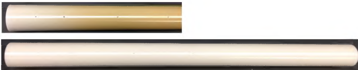
Figure 7.5: Waveguide color changes after heat treatment. Top: Color gradient indicates oxidization of the hottest area. Bottom: The whole sample became white after high temperature sintering at a uniform temperature distribution.
