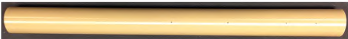
Figure 7.2: Yttria stabilized zirconia rod as received from Astro Met, Inc..
