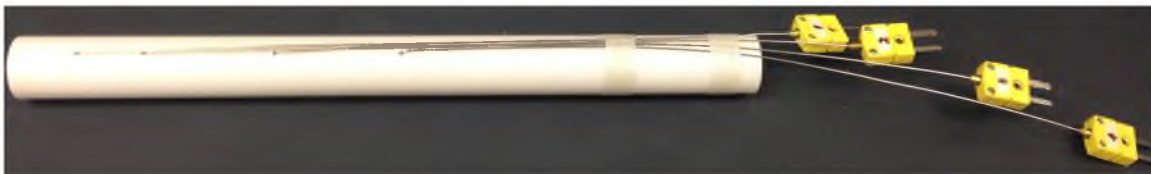
Figure 7.6: The placement of thermocouples used during real-time temperatures monitoring.
