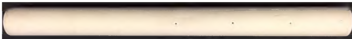
Figure 4.4: Three 3/32 -inch holes were drilled into the precast alumina rod at 2, 4, and 6 inches away from the distal end of the rod.
