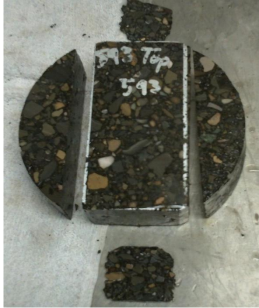
Figure 3 - Example of block being removed from circular puck
