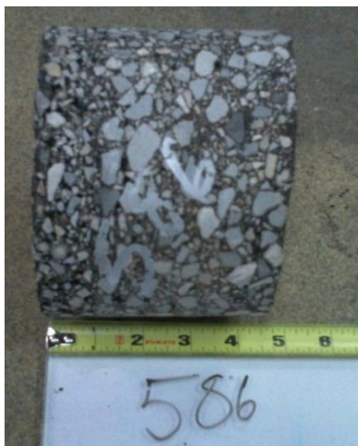
Figure 2 - Field core displaying multiple layers of asphalt concrete
