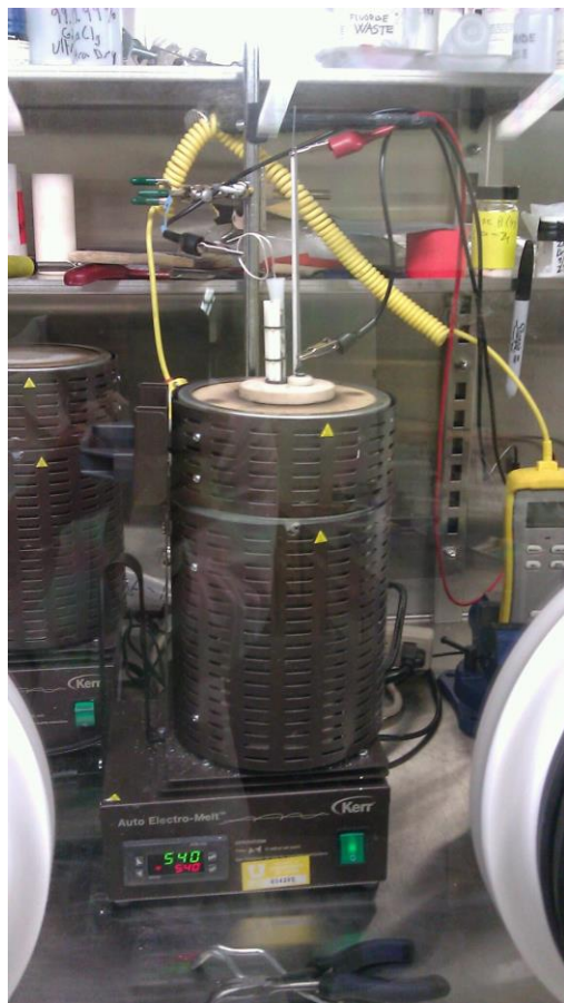
Figure 5.7: Kerr furnace operating within the glovebox.
