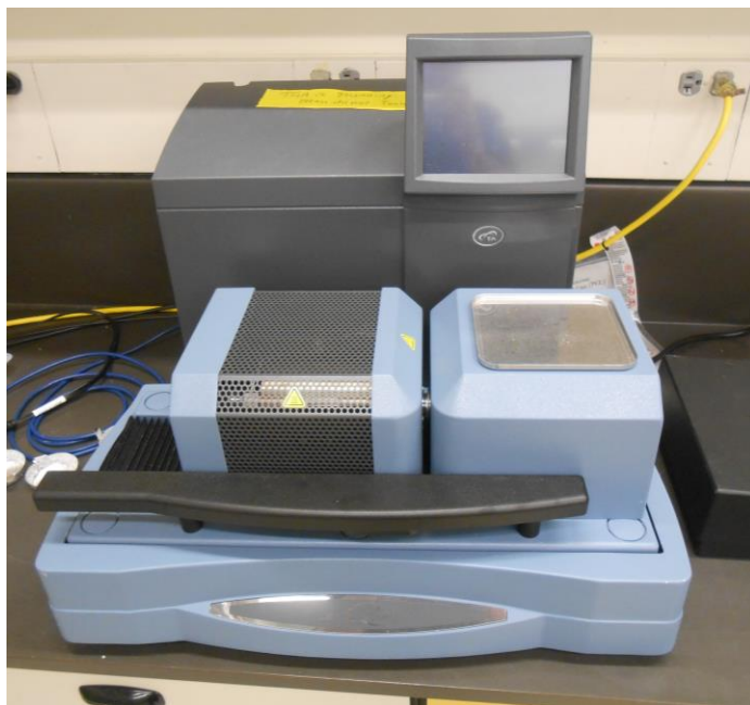
Figure 5.9: The DSC/TGA unit used for thermal analysis of salt samples. Samples were run to 923 K under the flow of ultrapure argon.
