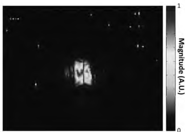
Figure 12. Demonstration of k-space spikes. The bright points on the edges of this k-space image could be the result of gradient cables that are not sufficiently tightened (123) resulting of electric arcing that is detected by the RF receive coils. In our experiments, tightening the gradient cables and implementing RF shielding was effective in removing the k-space spikes.
