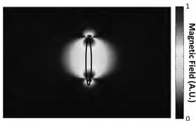
Figure 16. The magnetic field of a loop. The magnitude of the magnetic field perpendicular to the loop (outlined in black), created from the analytical solution of the magnetic field of a loop.
