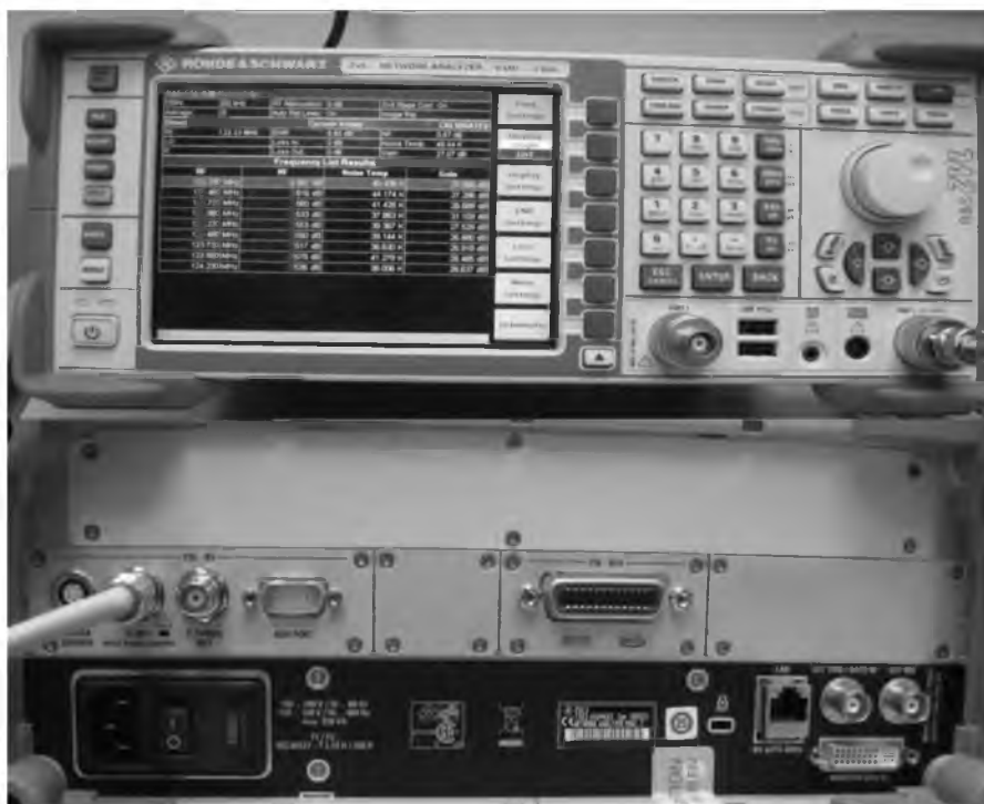
Figure 19. A Rhode and Schwarz Network Analyzer with noise figure meter option.
