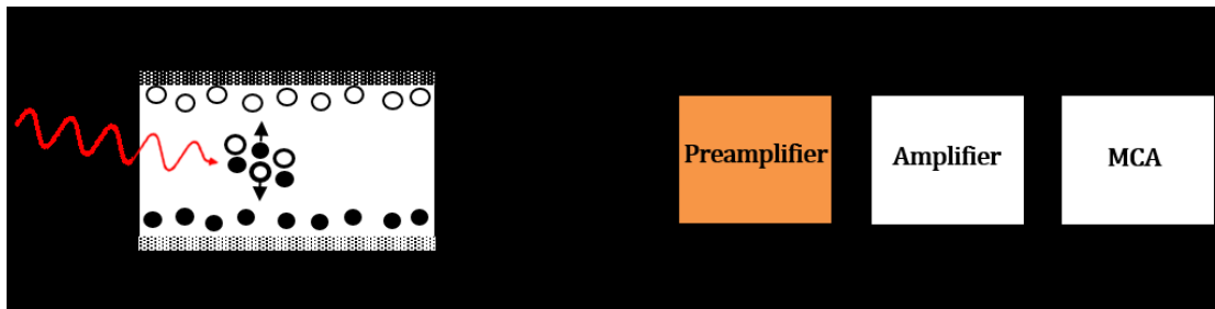
Figure 2-3. Schematic of semiconductor detector components used for \gamma -ray spectroscopy. Electron-hole pairs are created following excitation due to incoming \gamma -rays. High-purity germanium semiconductor detectors must be housed in a vacuum-tight cryostat and cooled to liquid nitrogen temperatures (77 K) to inhibit thermal conductivity between the detector crystal and its surrounding environment. In most cases, the detector crystal and preamplifier are unified, whereas the amplifier and MCA are separate units.
