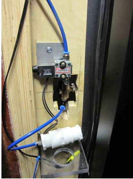
Figure 3. Nozzle and scent container mounted to the outside of the air inlets, with the scent lower than the nozzle.
