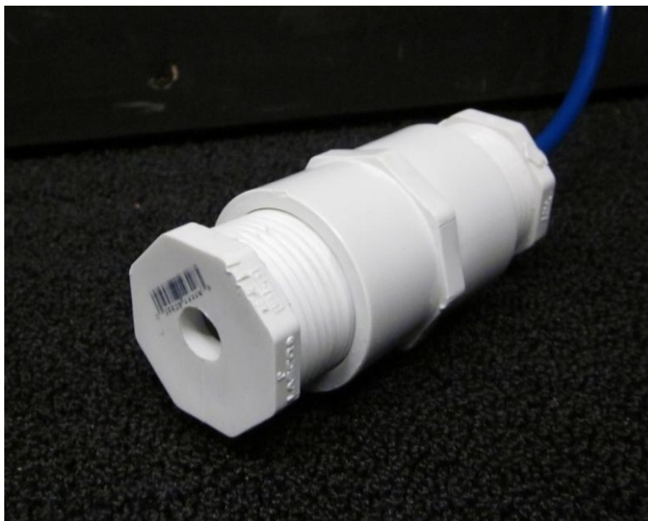
Figure 11. Scent container from a different angle, showing air inlet hole.
