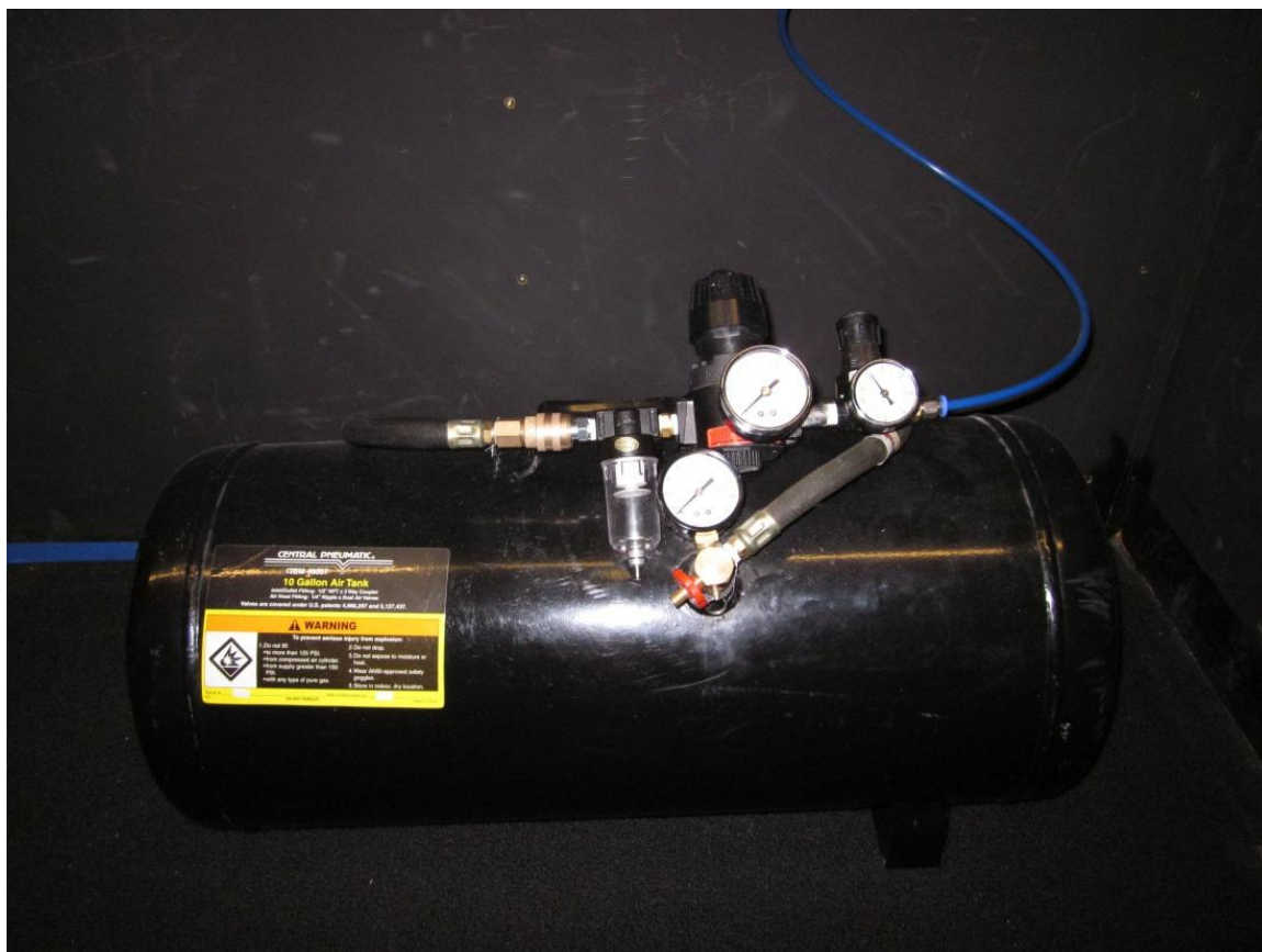
Figure 8. Ten gallon air tank.
