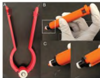
Figure 3 (A) The holder consists of two anchor arms, (B) The anvil tool with engaging ring, (C) A closer look of "Pushing the engaging ring".
