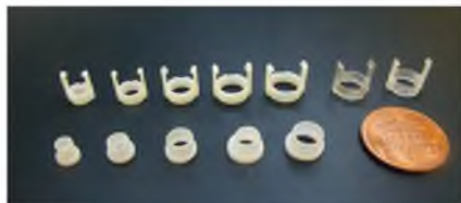
Figure 6 Engaging rings and back rings were manufactured in various sizes for vessels whose outer diameter ranges from 2mm to 6mm.
