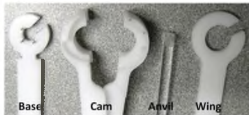
Fig. 3. The cam tool set showing the right base, cam, anvil, and wing closure tools.
