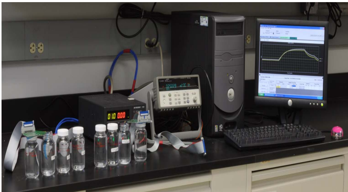
Fig. 5.4. Overview of the testing apparatus used to obtain sensor output characteristics. The sensor array was inserted into solutions of varying ionic strength and the output voltage signal was measured simultaneously [1].
