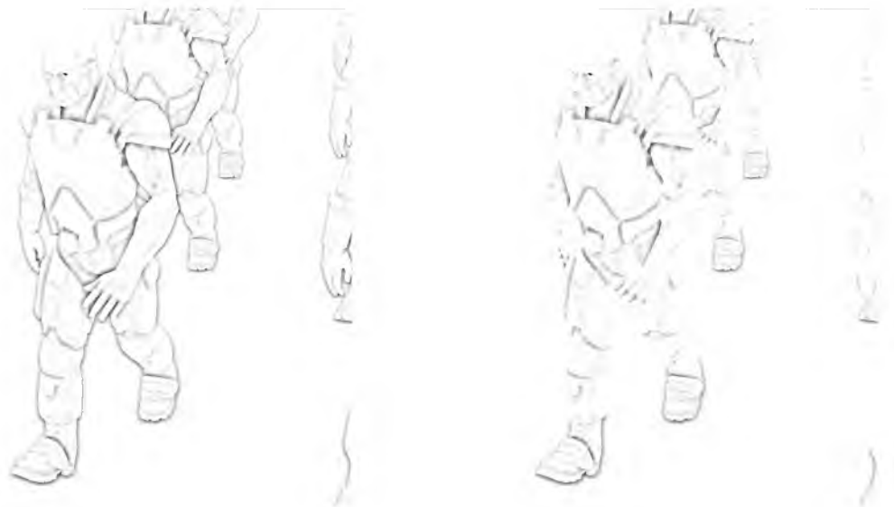
Figure 6.4: On the left thickness is not used (177 fps), on the right it is (163 fps). Notice how the silhouette edges are no longer shadowed when the thickness model is used.
