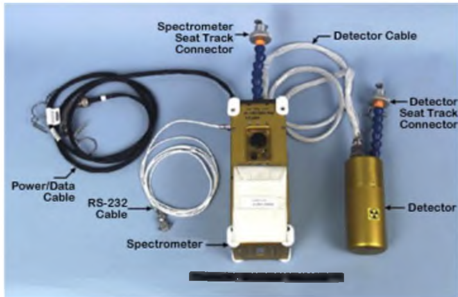
Figure 5.1: ISS Tissue Equivalent Proportional Counter, used by permission Space Radiation Analysis Group, Johnson Space Center, NASA [11].
