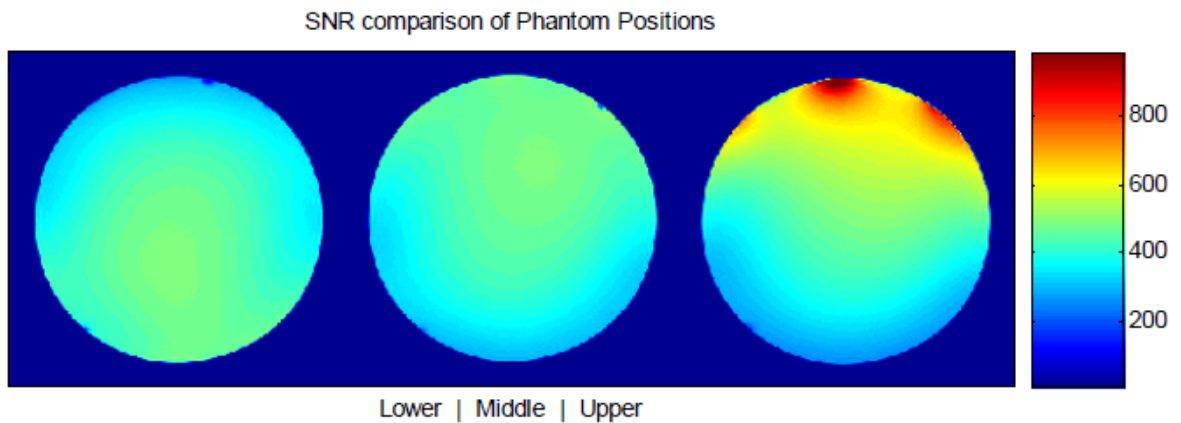
FIG. 4.12: Relative SNR plot of an axial slice through a cylindrical phantom placed in various locations within the Siemens 12-channel coil ( d_{\text{lower}} = 60\text{mm} , d_{\text{middle}} = 25\text{mm} , d_{\text{upper}} = 2\text{mm} ).
