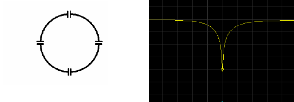
FIG. 2.45: A single resonant coil with an ideal resonant S_{11} curve.
