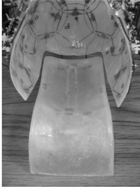
FIG. 3.7: Collapsible mask/headrest design (foam padding on headrest not shown).
