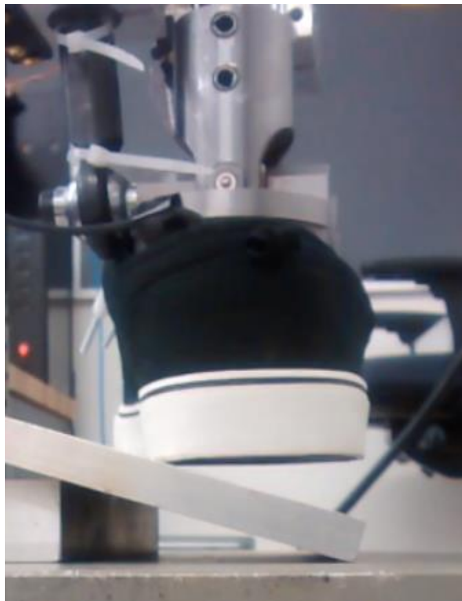
Figure 36: Ankle stiffness test setup.
