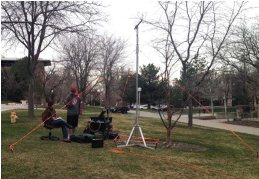
Figure 2.6: Photograph of the tower at location FASB2; note the CRDS in the wagon.
