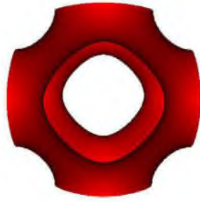
Figure 8.3. Isosurface constructed based on the analytical solution u(x, y, z) = \cos(2\pi x) + \cos(2\pi y) + \cos(2\pi z) for isovalue = 0.2 .
