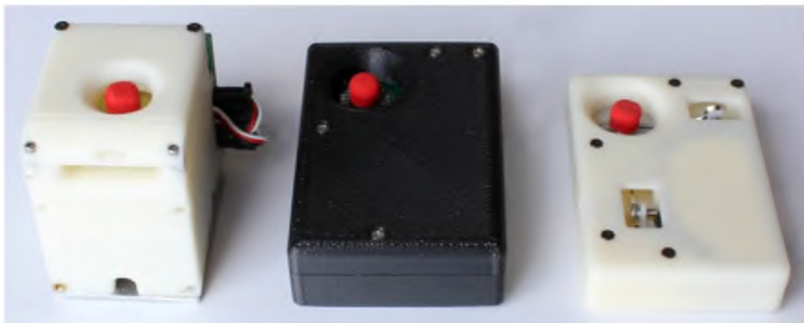
Figure 4.13 Form-factor comparison of (left) prior flexure stage design, (middle) LPSSD with embedded sensors, and (right) intermediate prototype without sensors.
