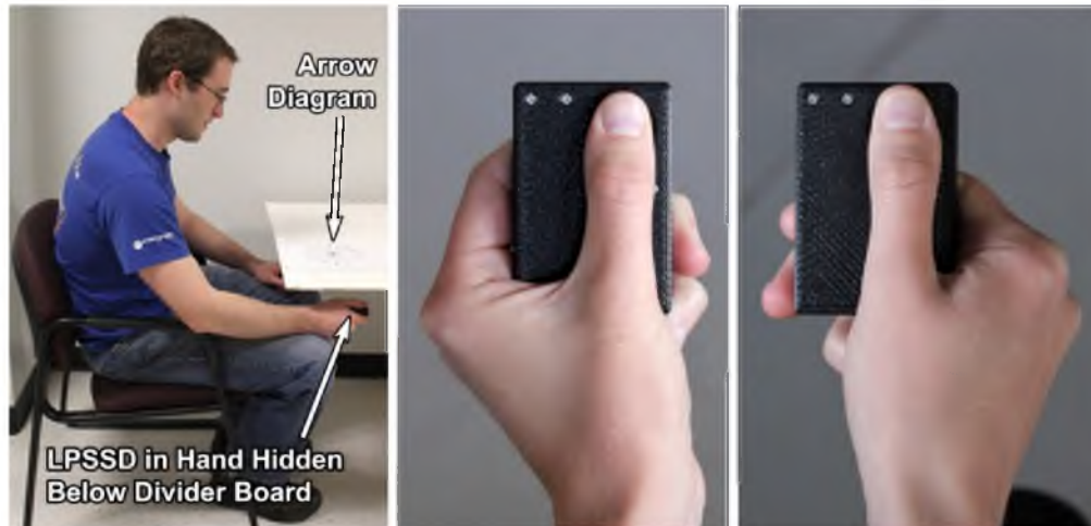
Figure 5.1 Test participant seating orientation showing the divider with arrow display obscuring the user’s view of his hand (left). Straight grip used for left hand pilot test (center). Straight grip used for right hand pilot test (right).
