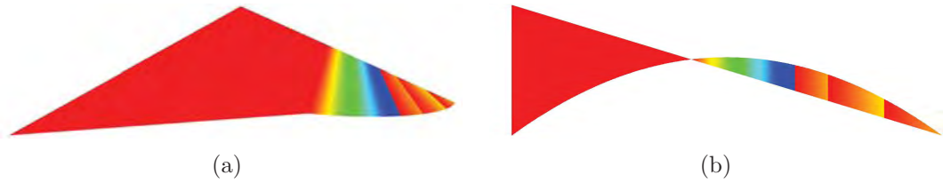
Figure 7.7. Views of Case 4 (negative Jacobians in a single tetrahedron) rendered with ElVis. Colors show Jacobian values from -0.5 to 0.0. Left is a view of the x + y + z = 1 face being intersected by the x - y face. Right is a view of the x - z face, where the self-intersection effect of the quadratic node at (0.5, 0, 0.6) is apparent.
