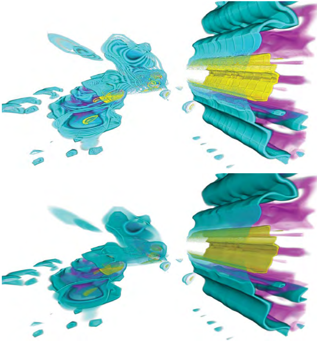
Figure 6.5. Image quality comparison between Riemann sum evaluation (top) and our algorithm (bottom) for the block and splitter plates data set. Both images were generated using 140 million samples and rendered in two seconds for a 1600 \times 800 image. Notice the banding present in the top image, which is an indication of insufficient sampling resolution.
