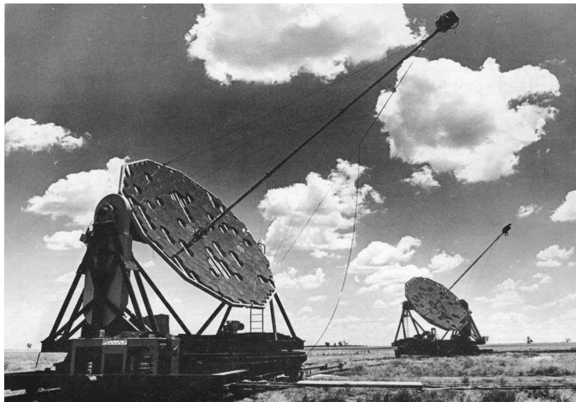
Figure 1.1. Light collectors used in the Narrabri stellar intensity interferometer. Image from Sky & Telescope , vol. 28, pp. 2-7, 1964.
