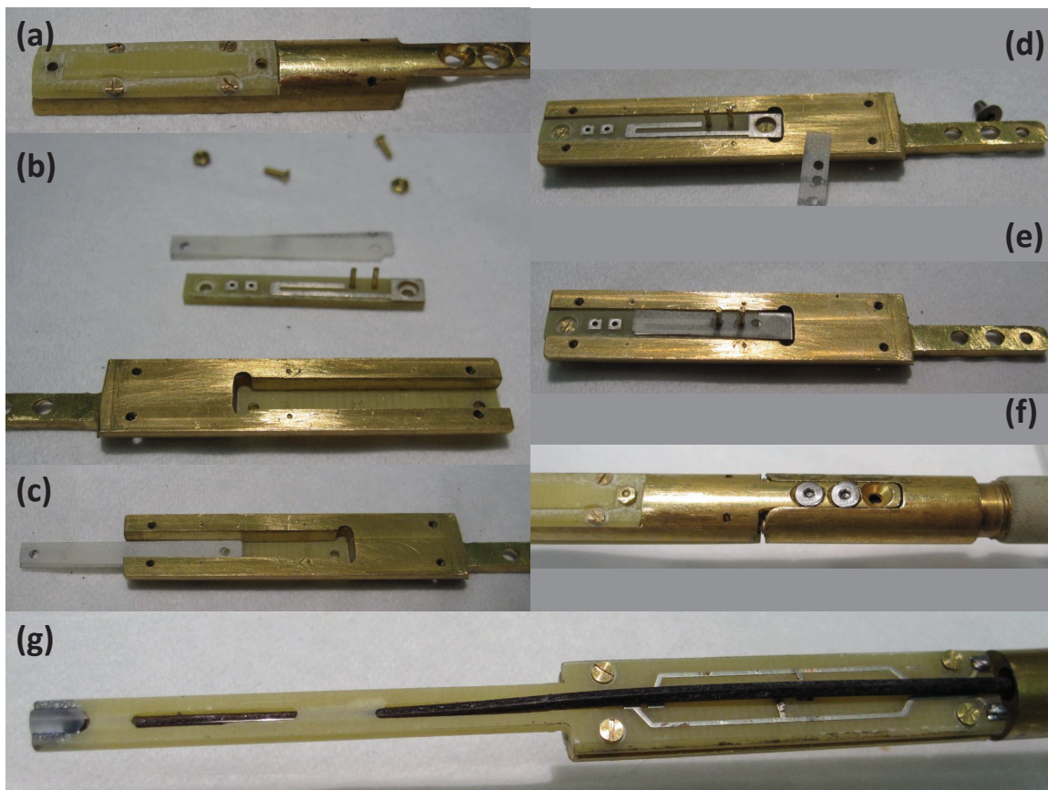
Figure A.4: Assembling procedure of EODMR sample holder, which is combined with three kinds of PCBs and a tuning fork shaped brass part. For details see text.
