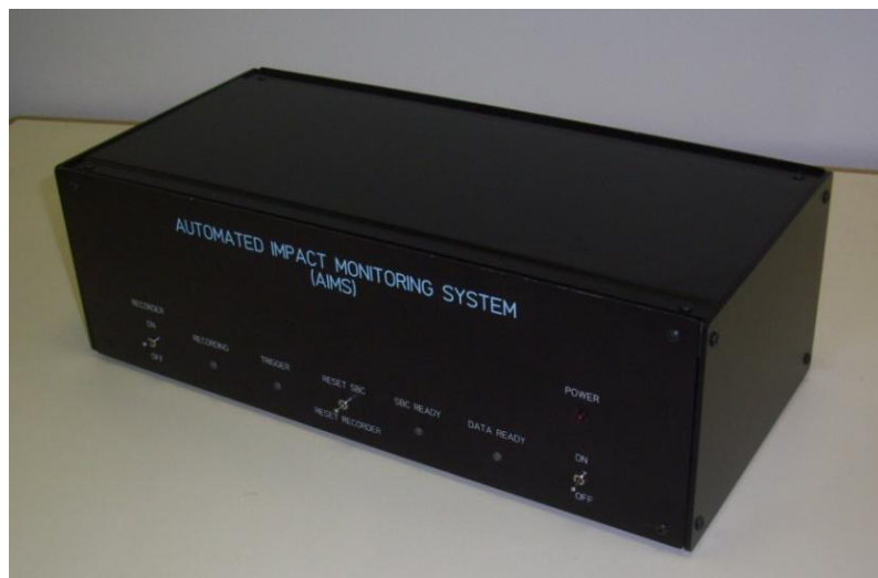
Figure 37. Automated Impact Monitoring System (AIMS) developed by Digital Wave Corporation in conjunction with ATK.
