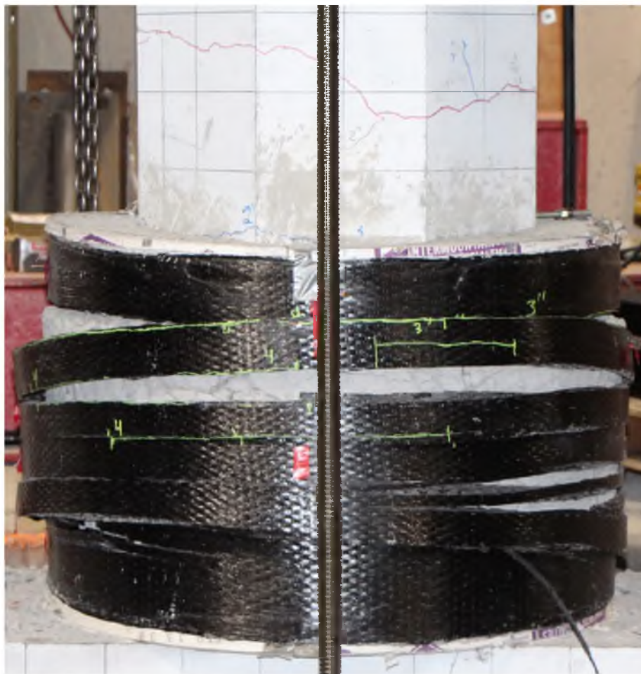
Figure 121. PCLen-3R Final Damage
