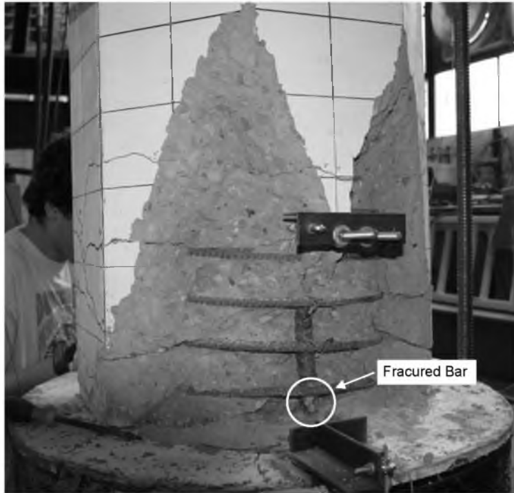
Figure 103. PCLen-2R East Face Final Damage
