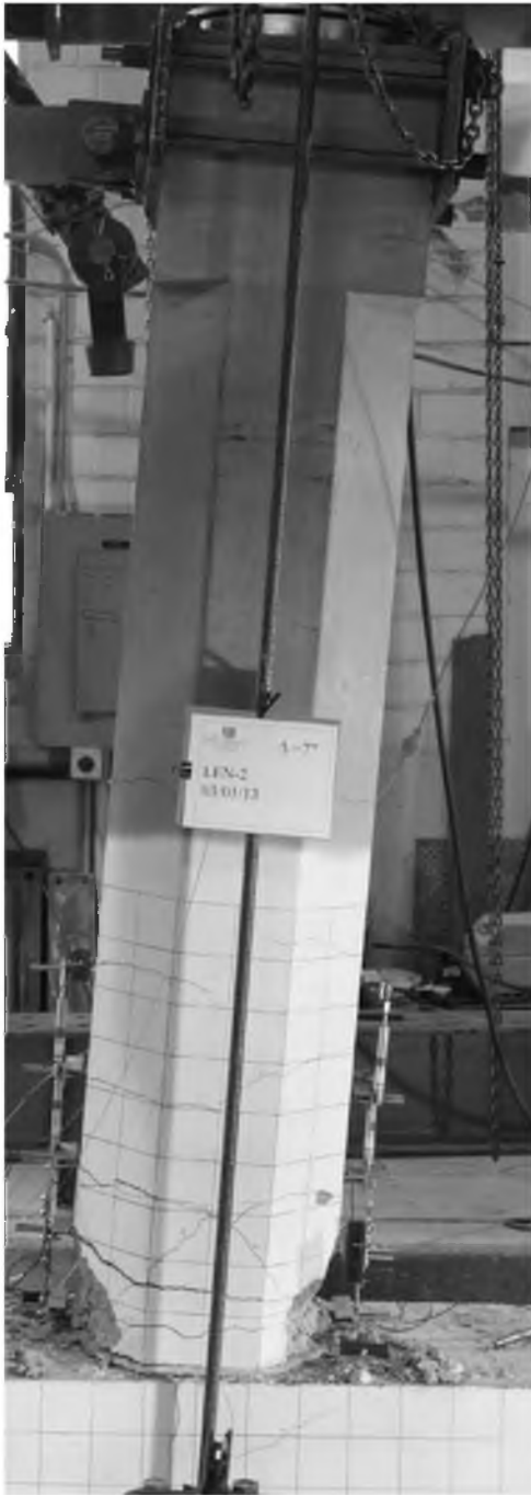
Figure 102. Test Comparison (a) PCLen-2 at Maximum Drift (b) PCLen-2R at Maximum Drift
