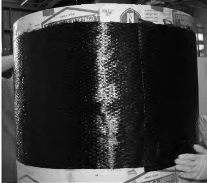
Figure 85. Prefabricated CFRP Shell on Sono Tube Form
