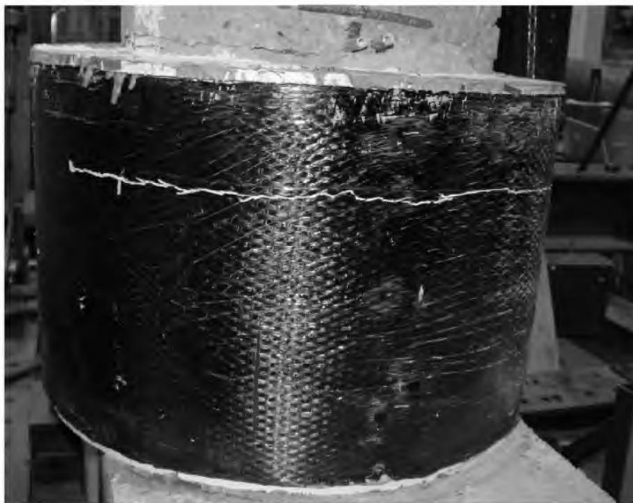
Figure 106. PCLEN-2R Transverse CFRP Crack
