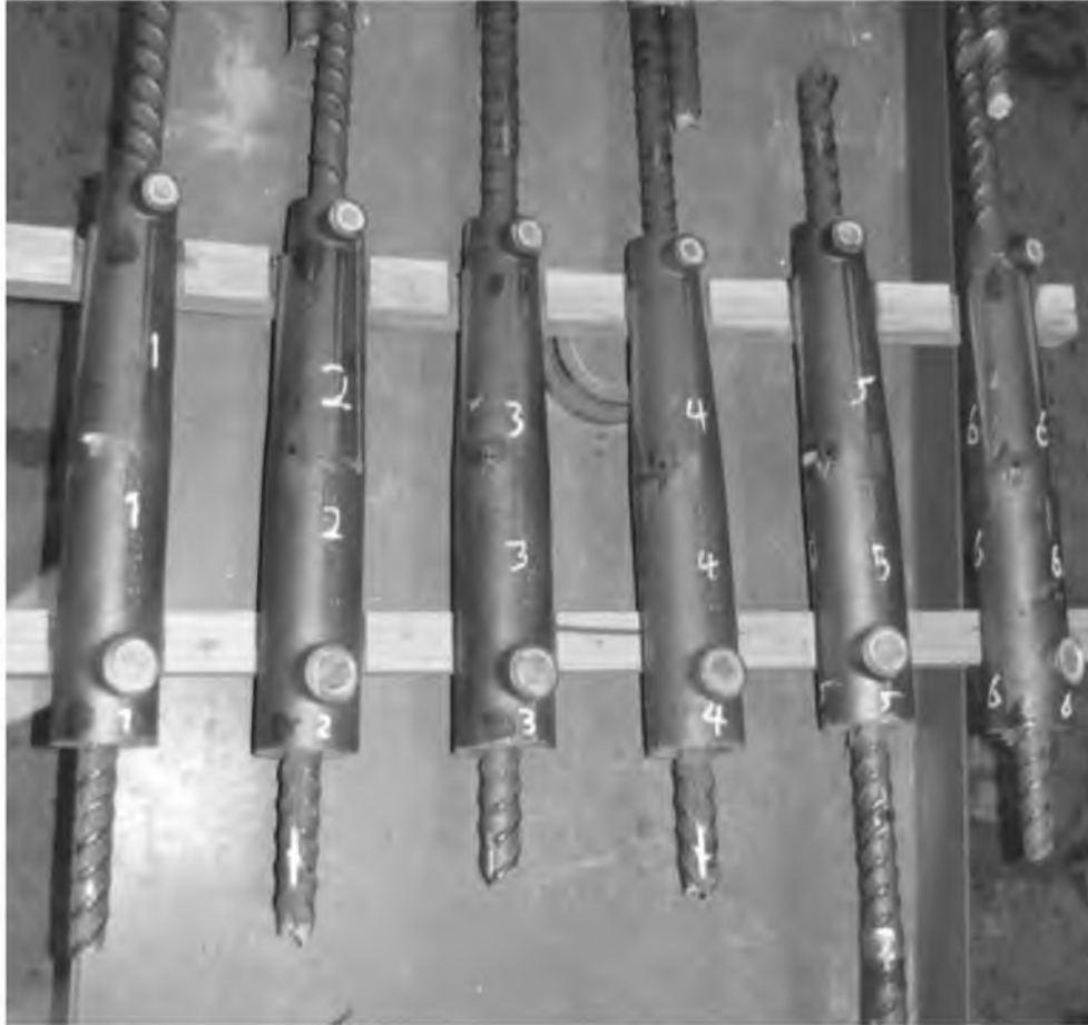
Figure 22. NMB Splice Sleeve Failure Mode
