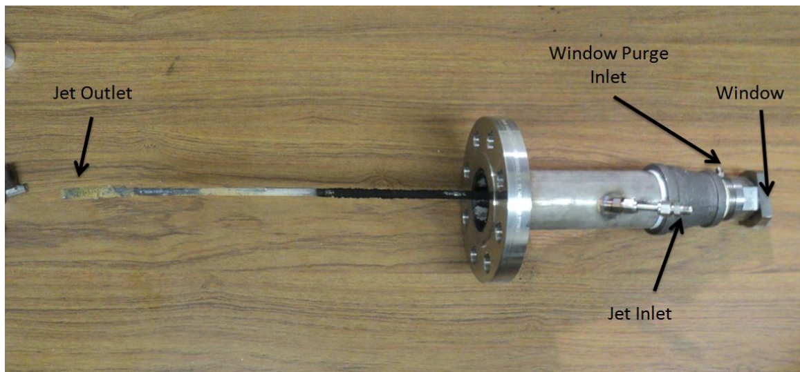
Figure 4.17. Jet diversion device. The major features of the device are labeled. The unit was mounted in the sample port on the gasifier.
