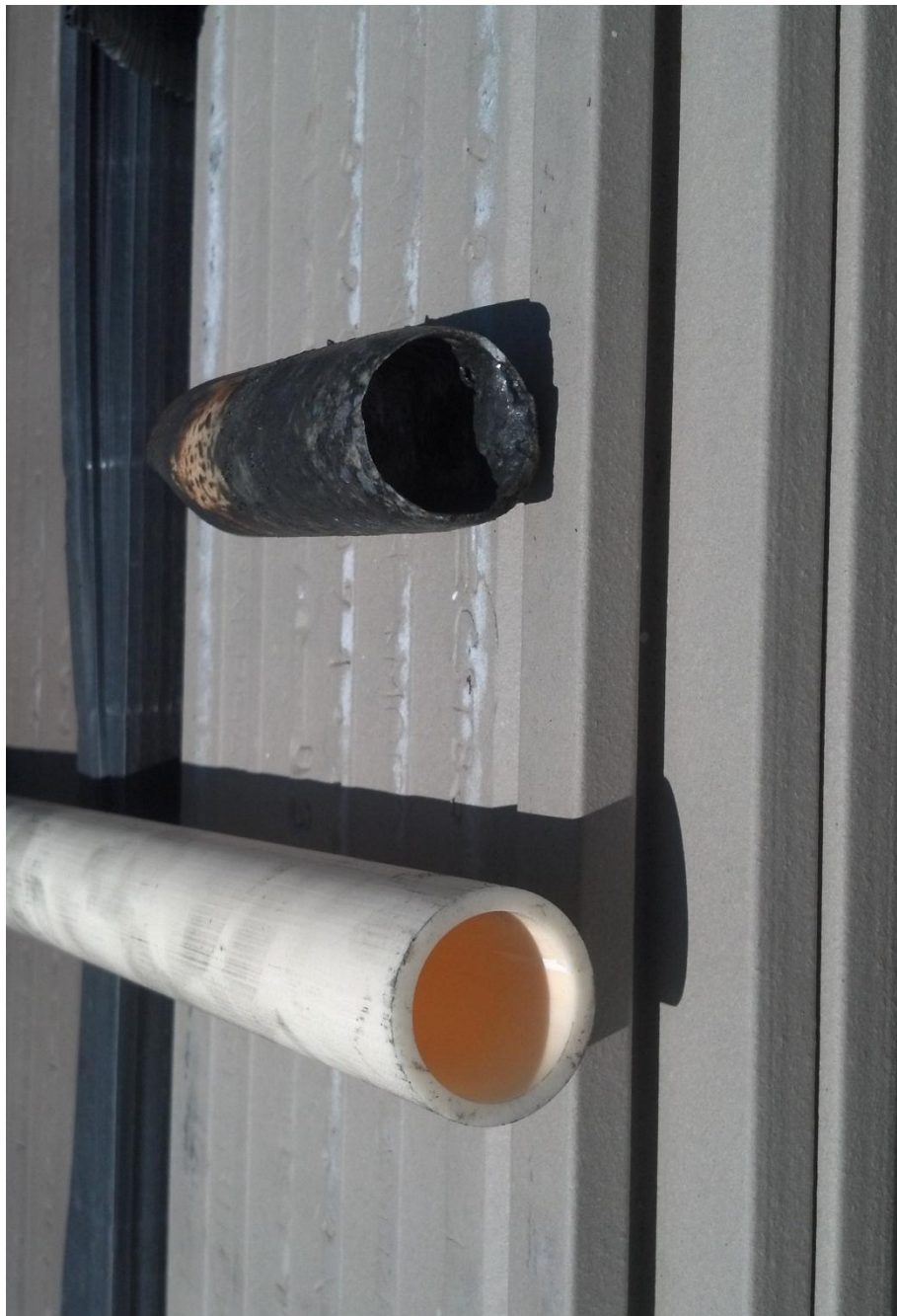
Figure 5.31. Recovered alumina tube from gasifier experiments. Also pictured is an unused alumina tube for visual comparison. The used tube was eroded when exposed to the gasifier. The top of the tube suffered a much higher rate of erosion than the bottom, losing nearly 2.0 mm of thickness in just 20 hours of exposure to the gasification environment. Some unreacted carbon can be seen in the bottom of the used tube.
