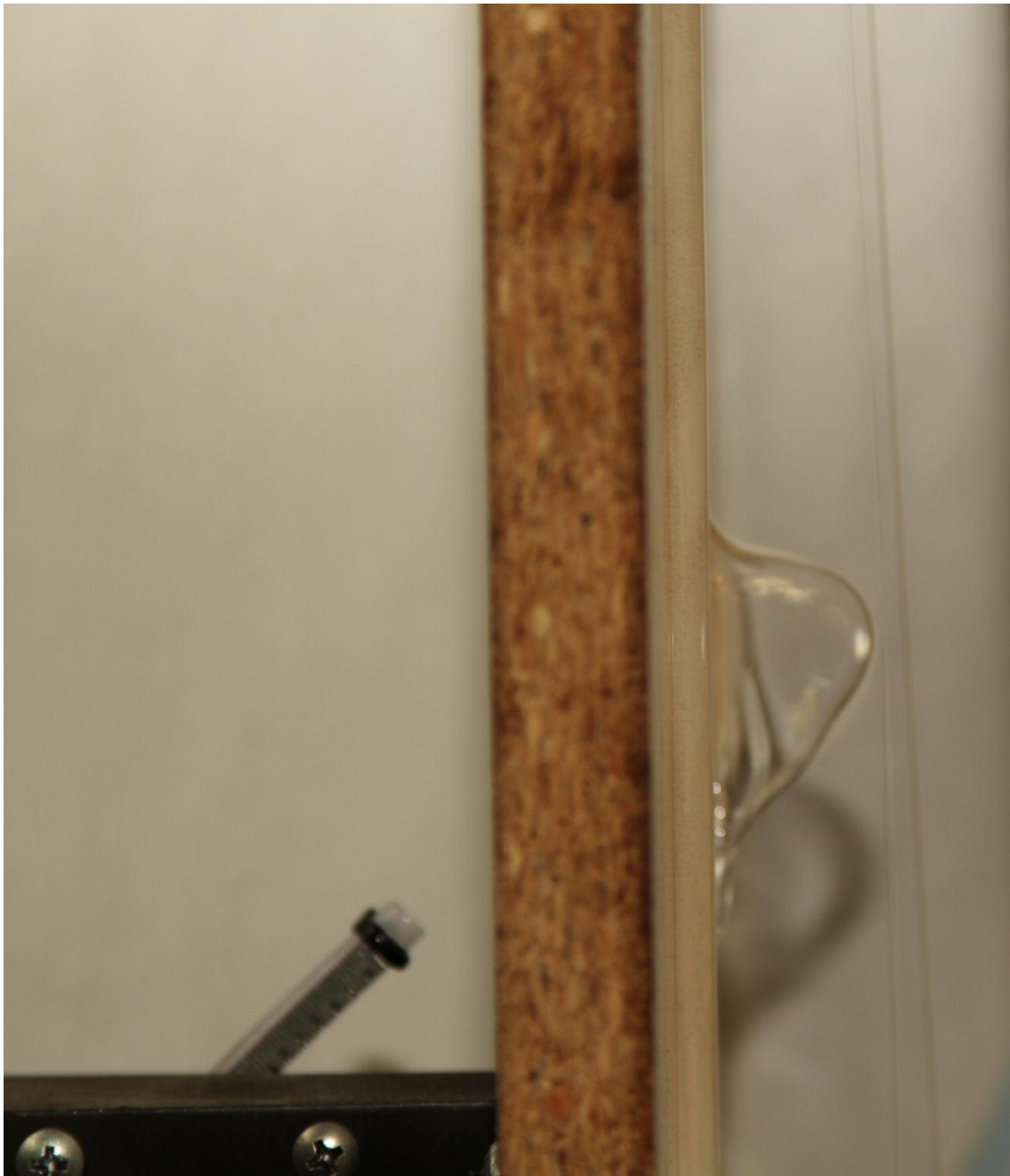
Figure 5.5. The reformed oil bubble. In this photograph is 12,500 cSt silicone oil film, after the gas jet flow rate was decreased to 0.22 g/s. At this flow rate, the hood formation has dropped across the jet stream and reformed the film.
