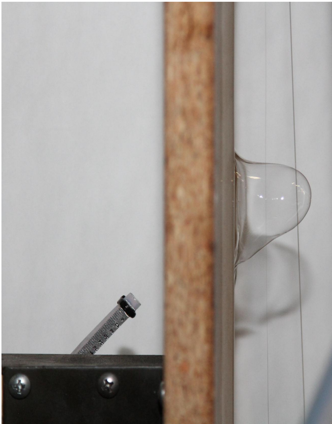
Figure 5.2. Higher flow gas jet with increased bubble size. This photo is of the same 12,500 cSt film as Figure 5.1 with an increased jet flow rate of 0.25 g/s. The bubble has pulled even farther away from the film.
