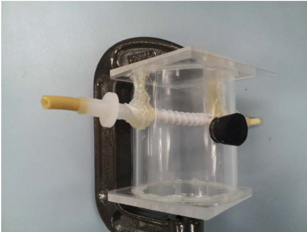
Figure 12. Mylar sheets curing. The graft placement slots are being filled with silicone (although this model does not show thermocouples).
