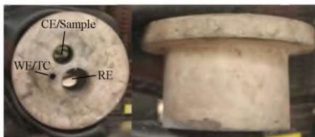
Figure 3.5: Top (left) and side (right) view of alumina plug
