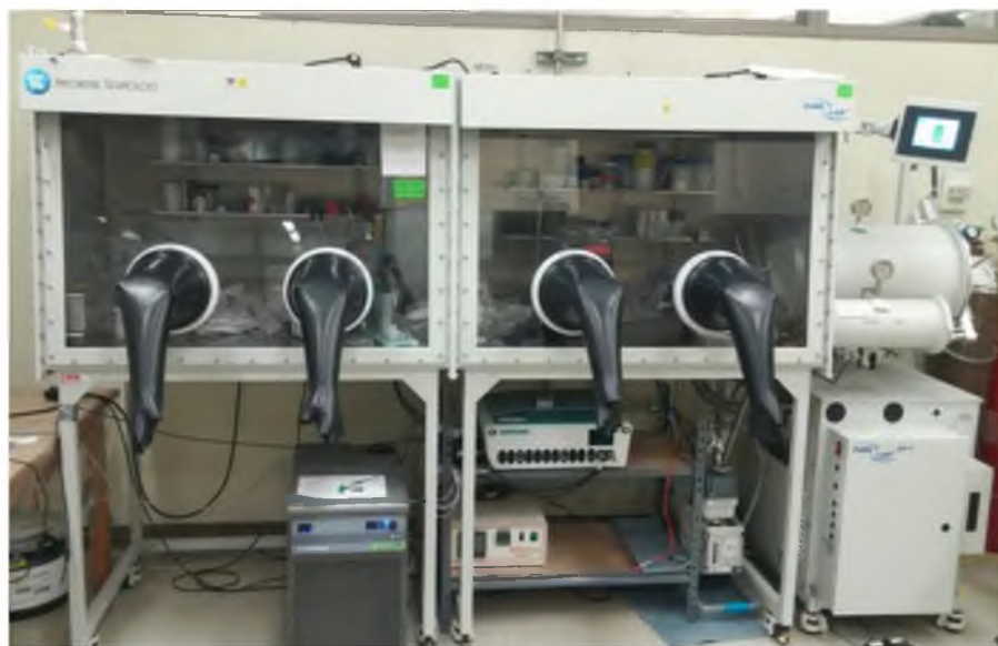
Figure 3.3 Picture of glovebox in which electrochemical test were conducted
