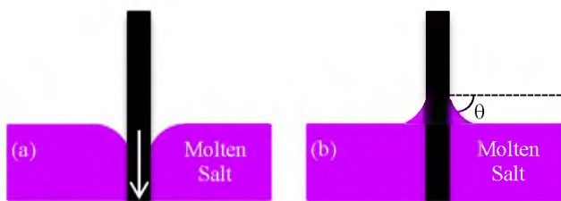
Figure 3.8 Illustration of surface tension effect for (a) immersing WE into salt and (b) wetting on a static WE
