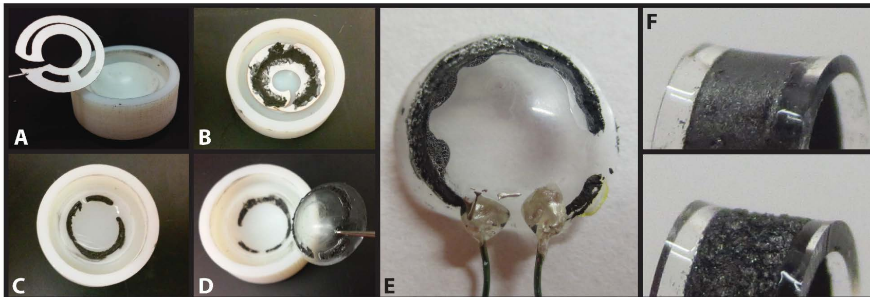
Figure 4.2. Contact lens biofuel cell fabrication steps. (A) A laser-cut electrode tape mask is placed in the mold, (B) carbon paste is applied over the mask, (C) the mask is removed revealing the patterned carbon paste electrodes, and (D) UV-curable elastomer is poured over the electrodes and cured while the mold is spinning to produce the lens with electrodes molded into them; (E) shows the finished device with leads attached to it; (F) carbon paste electrode surface area increased when the carbon paste was transferred to the lens material before the paste fully cured.
