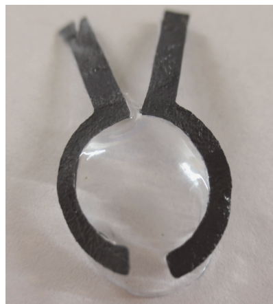
Fig. 2. Contact lens biofuel cell prototype including the connection leads.
