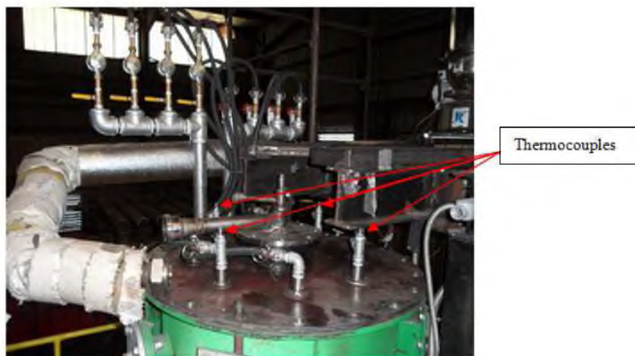
Figure 41. Position of thermocouples on top plate
