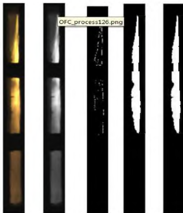
Figure 44. Procedure of optical methodology to measure flame stand-off distance
