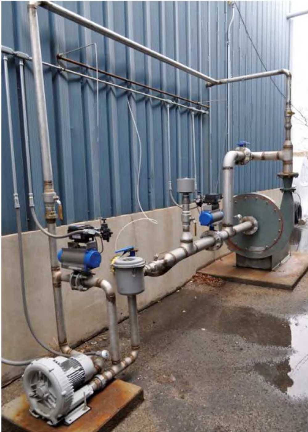
Figure 9. Recycle Flue Gas system of OFC at University of Utah
