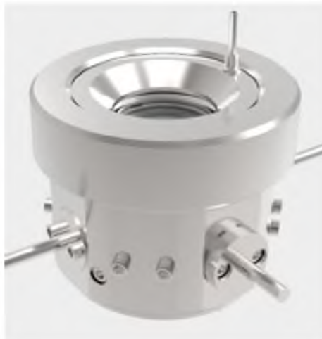
Figure 2.5. A piston cylinder style DAC designed for resistive heating, capable of reaching temperatures of \approx 1000 K. Pressure is applied by means of four pressure screws which engage the piston via through-holes in the cylinder, or through the use of a steel membrane which is attached to the cylinder directly and applied pressure when inflated with gas. This figure shows the Helios DAC, which is designed for high temperature. Many measurements in the works were also taken using the Diacell Bragg DAC. The styles and alignment of the two are very similar. The bottom seat is secured to the cylinder with four set screws, allowing for lateral adjustment. The top seat is affixed to the cylinder by means of three set screws on a rocker, which allows for very fast and accurate tilt adjustment. Both DACs provide pressures >100 GPa using 200 \mu\text{m} diameter culet; pressures of \sim 50 GPa are routinely achieved. The pressure drift with temperature in the piston-cylinder type DAC is generally not great \pm 2 GPa, except in the case when the helium membrane is employed when cooling to low temperatures. In this case, the pressure tends to increase by very noticeable amounts of >5 GPa. Picture courtesy of Alamx-easylab.
