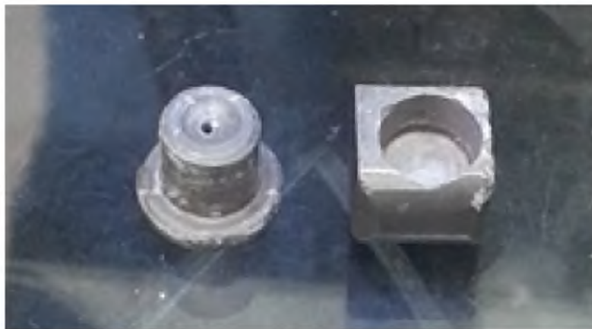
Figure 7.2. Modified crucible used to grow single crystals of lithium. Crucible and plunger are machined from Mo. The hole in the plunger was made using an EDM; the hole is \approx 500 \mu\text{m} and tapers to \approx 200 \mu\text{m} hole at the top. The size of the crucible is \approx 0.75 \text{ cm} .
