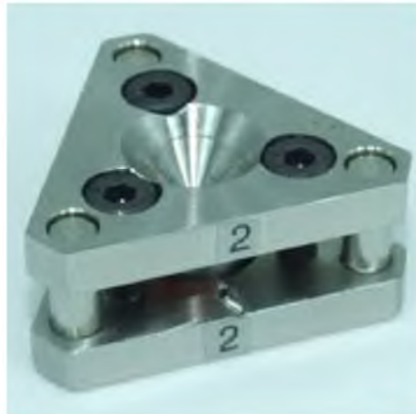
Figure 2.4. Another style of plate DAC; this is a miniature model manufactured by HPDO (hpdo.com). The pressure is applied by means of the three pressure screws. The posts attached to the bottom plate fit snugly into the top plate and preserve the diamond alignment as pressure is applied by gently tightening each screw separately. Both seats are attached to the plate by means of set screws, allowing for lateral adjustments. The only mechanism to adjust the tilt is by properly epoxying the diamonds; see section 2.1.1.
