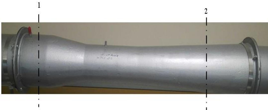
Figure 4.2 Two different sections of venturi-tube
