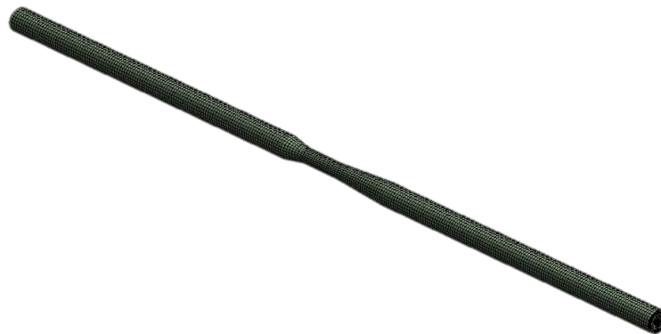
Figure 4.5 Surface mesh of venturi-tube
