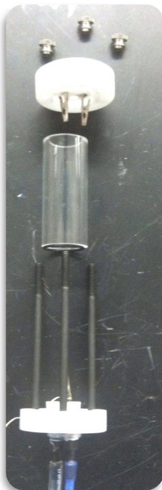
Figure A.5. Picture of the initial test cell used for experimental testing disassembled.
