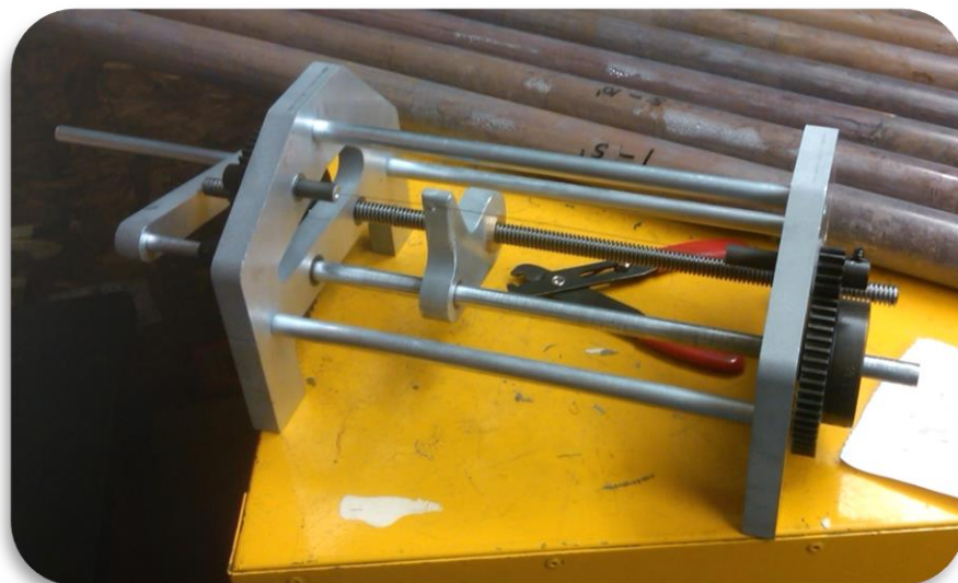
Figure A.2. Picture of coil winder mechanism used for metal coil creation.
