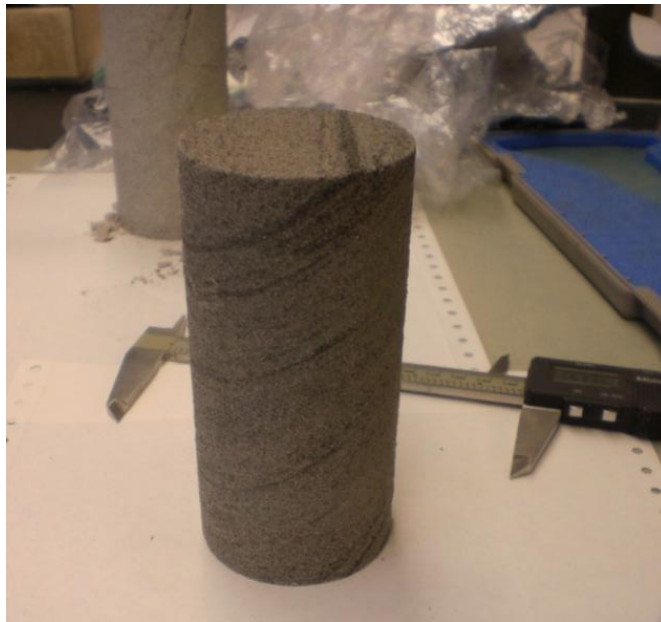
FIGURE 4.3 Photograph of a prepared cylinder of the channel sandstone material
