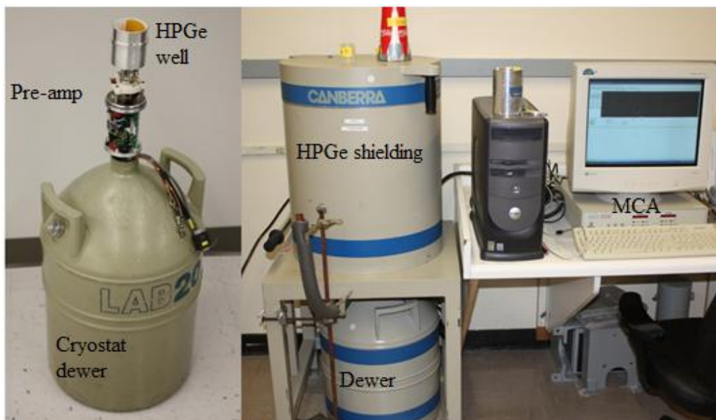
Figure 2-7 Nonshielded and shielded HPGe detectors at UNEP
