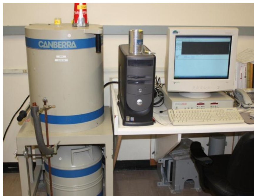
Figure 3-4 UNEP NAA station with GC-4020 HPGe, DSA-2000 MCA and computer system (Counting Station #8, UNEP as of 2012)
