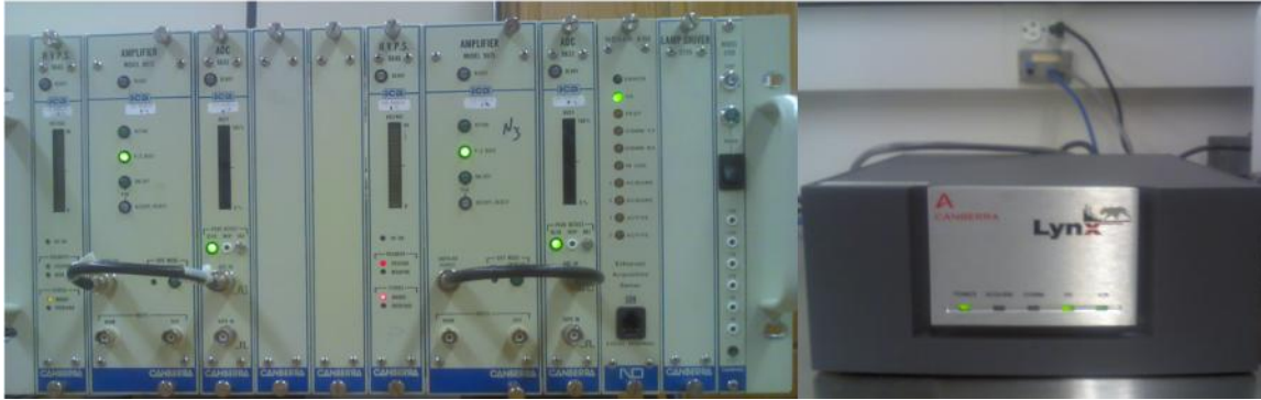
Figure 2-9 Canberra NIM based MCA and Lynx MCA as found at UNEP in 2012
