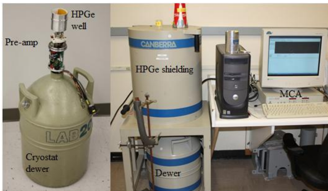
Figure 1 Non-Shielded and Shielded HPGe Detectors at UNEP
