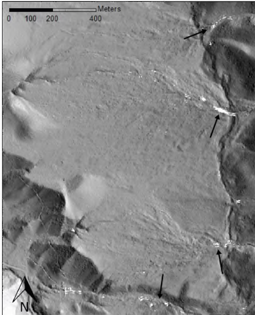
Figure 8: Hillshade map with black arrows denoting holes in the DEM caused by overly aggressive filtering of the LiDAR point cloud. The holes contain no data and therefore reflect the background color of the display screen.
