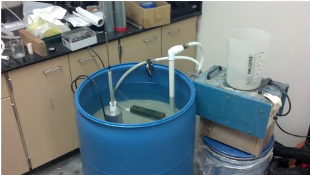
Figure 1.8. 55-gallon seepage drum showing peristaltic pump, well screen pump return, and installed Shelby tube with amplifier.
