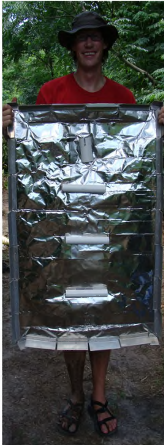
Figure 2.2. Photo displaying stainless steel foil bottom of the seepage blanket. Author for scale.
