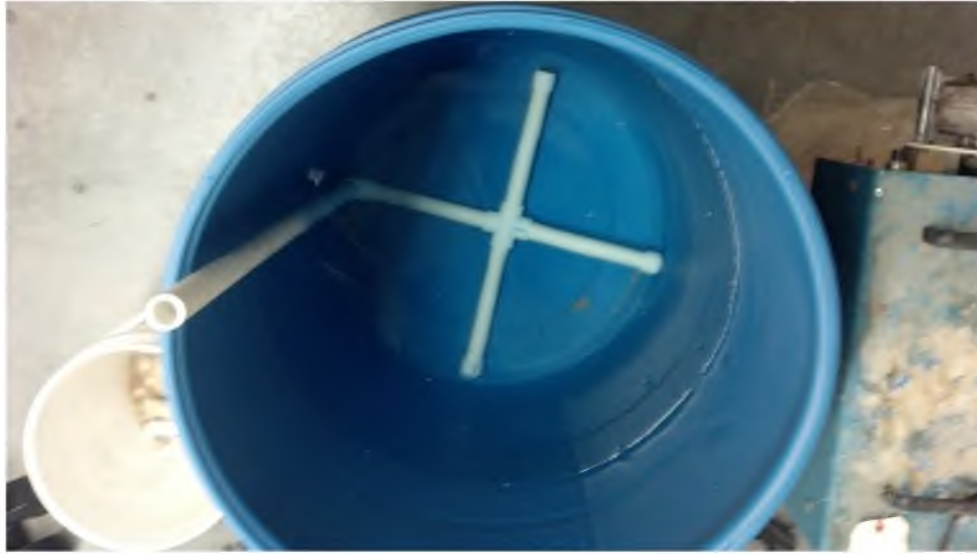
Figure 1.7. PVC pipe and well screen use to direct water to the base of a 55-gallon drum.
