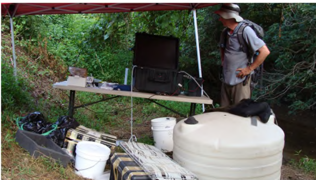
Figure G.3. Photo of injection site showing pump setup and stock tank holding NaBr tracer solution.
