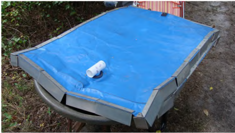
Figure 2.1. Seepage blanket showing rubber material construction, outlet port, and metal edging.
