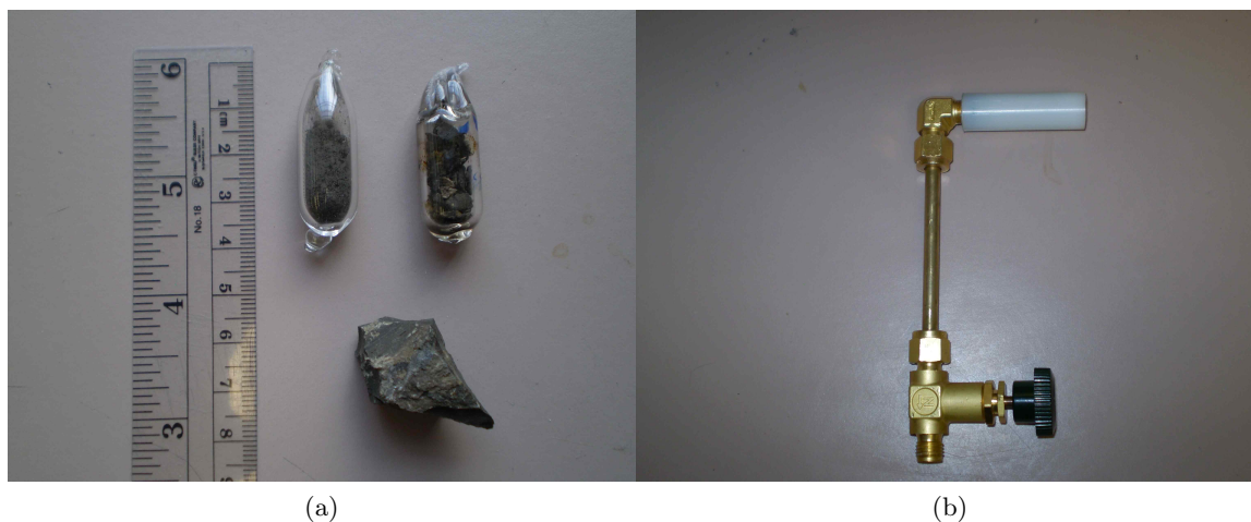
Figure A.2: Typical oil shale samples for high pressure work. (a) Upper - glass cells were used to contain the samples in the presence of a few atmospheres of gas. Lower - a typical sample of bare shale for use in the high pressure cell shown in Fig. A.1. (b) Samples for use in the 8 T xenon gas measurements.
