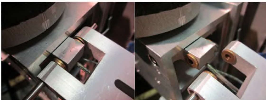
Figure 6.2 Quick release hinge connecting arm support linkage to force sensor housing. Shown connected (left) and disconnected (right).
