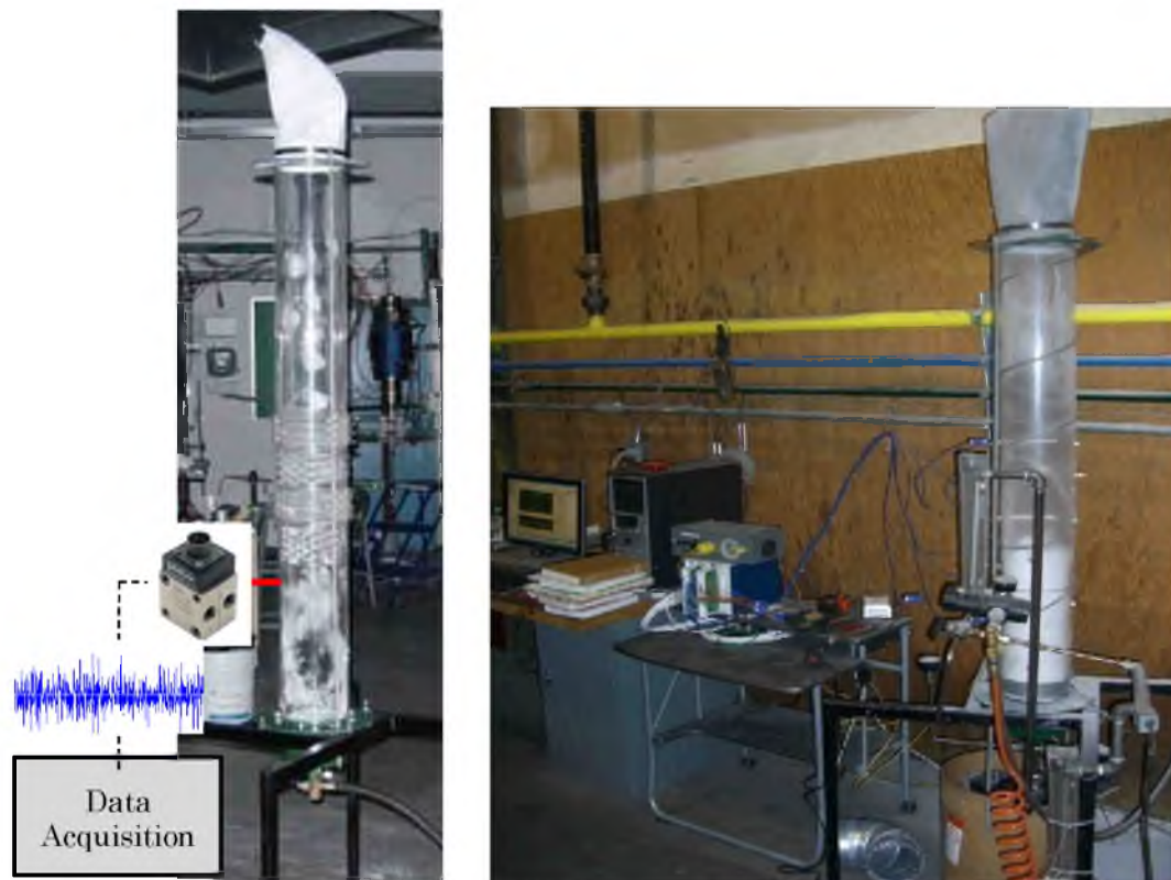
Figure 10. Cold-flow fluidized bed apparatus and pressure transducer assembly diagram
