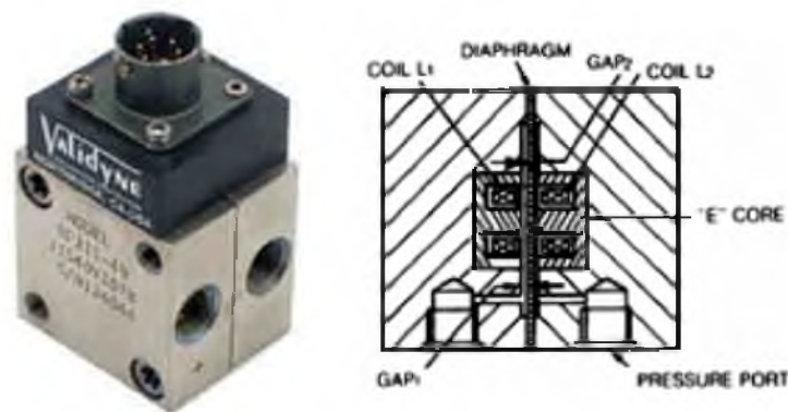
Figure 9. Validyne DP15 differential pressure transducer
