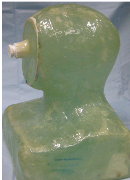
Figure 1. Head, neck and shoulders phantom. Custom fiberglass phantom filled with homogenous copper sulfate solution. This phantom was used for non-human rSNR comparisons.
