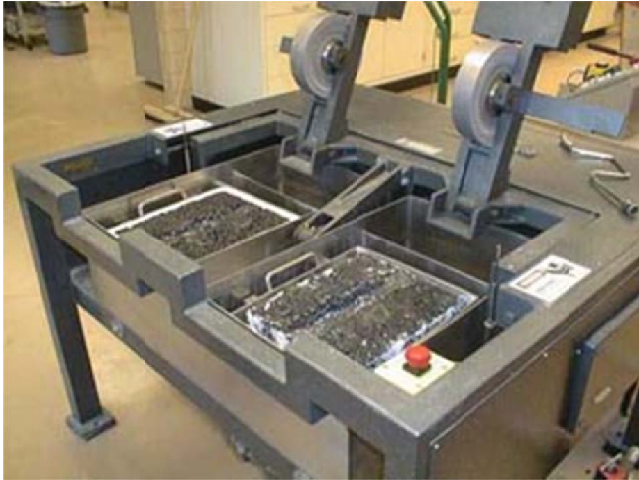
Figure 6- Hamburg Wheel Tracking Device
