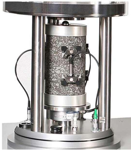
Figure 10- AMPT Testing Specimen
