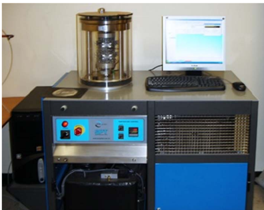
Figure 9- Asphalt Mixture Performance Tester
