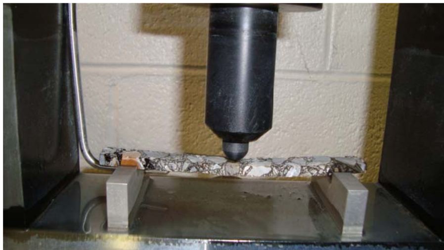
Figure 8- BBR Loading Set-Up (Outside of Liquid Bath)
