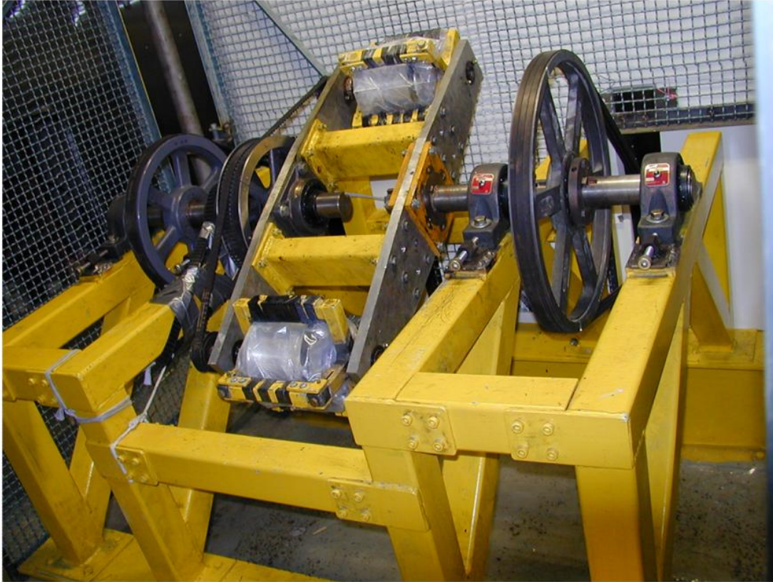
Fig. 4. 1 The dual drive planetary ball milling machine for nanoparticle production
