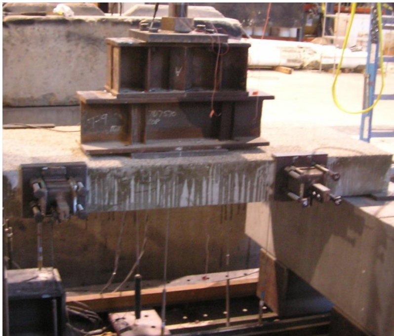
Figure 5.2: Posttensioned 3 ft Composite Specimen Under Cyclic Loading; (1 ft = 0.305 m)
