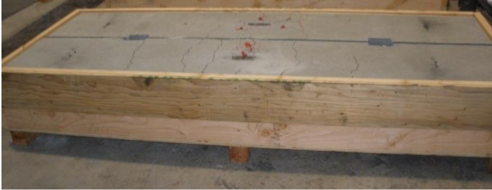
Figure 4.3: Type I Specimen Prior to Grouting and Placement of Overlay
